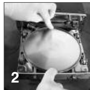
Press O-ring in at 6 and 12 o'clock.
