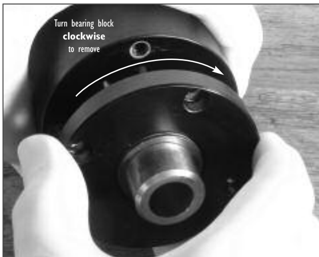
ACME thread on actuator stem is left-handed
