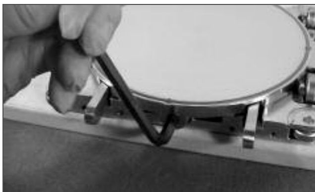
Remove set screw to access the gate spring
