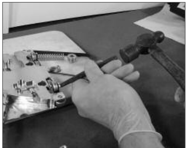
Use a punch and hammer to remove wheels from pins
