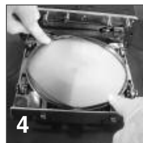
Continue pressing O-ring into groove at 180°-apart intervals.
