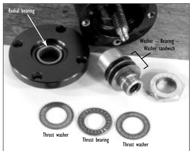
Drive nut and bearing block assembly parts
