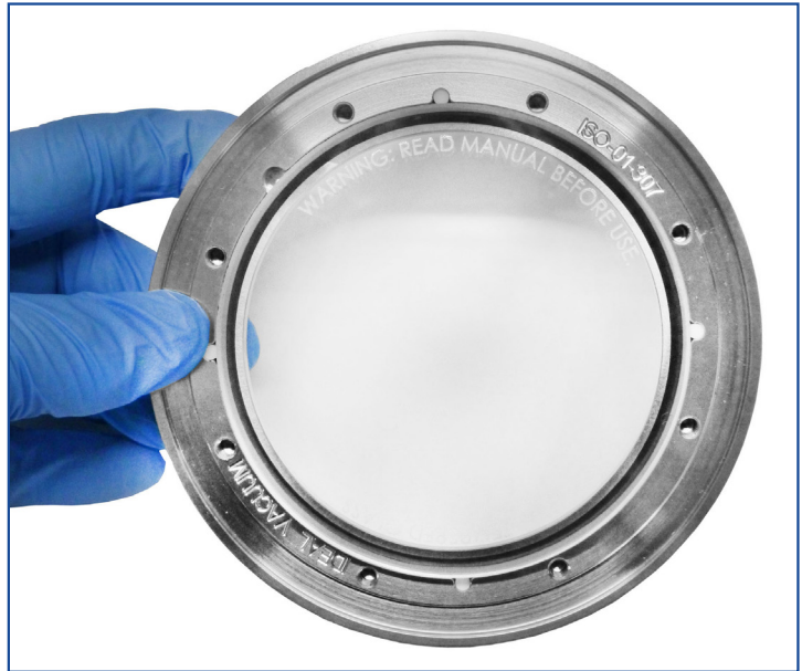
Figure 7 - Window pane placed onto flange
