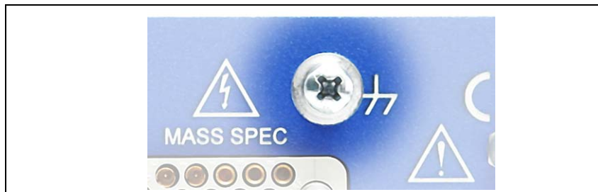
Figure 3-14 Ground Connection on the Rear of the VQM Controller
