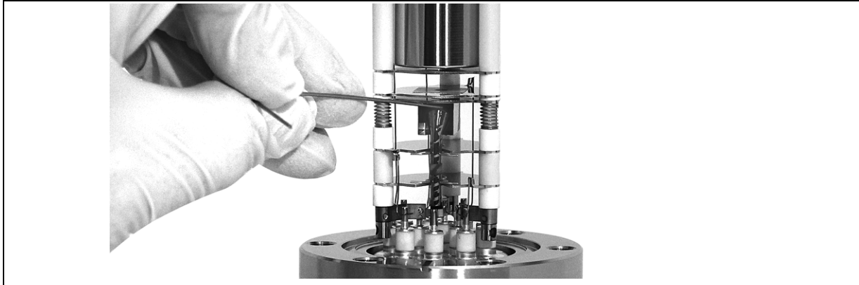
Figure 7-12 Electron Multiplier Adjustment
