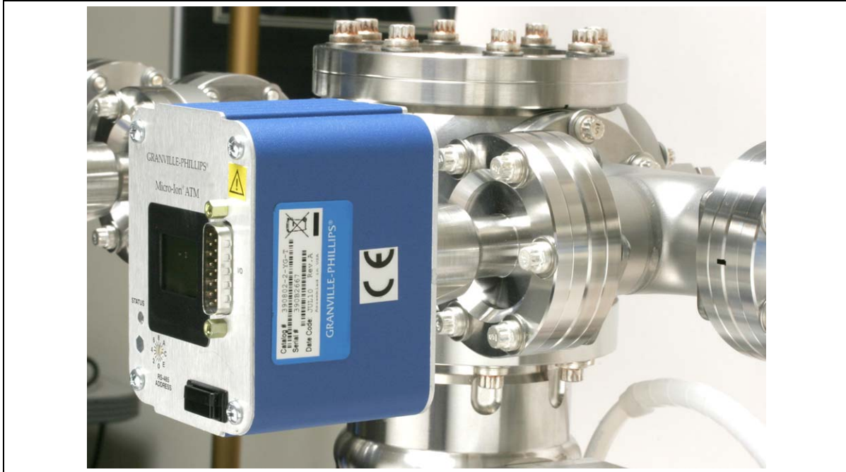
Figure 3-6 Micro-Ion Gauge Mounted on a Vacuum Chamber
