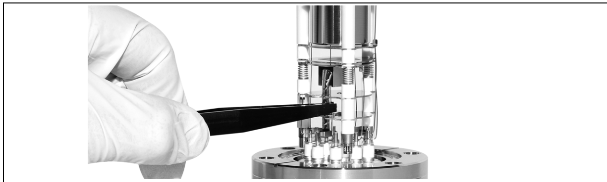
Figure 7-11 Remove the Electron Multiplier
