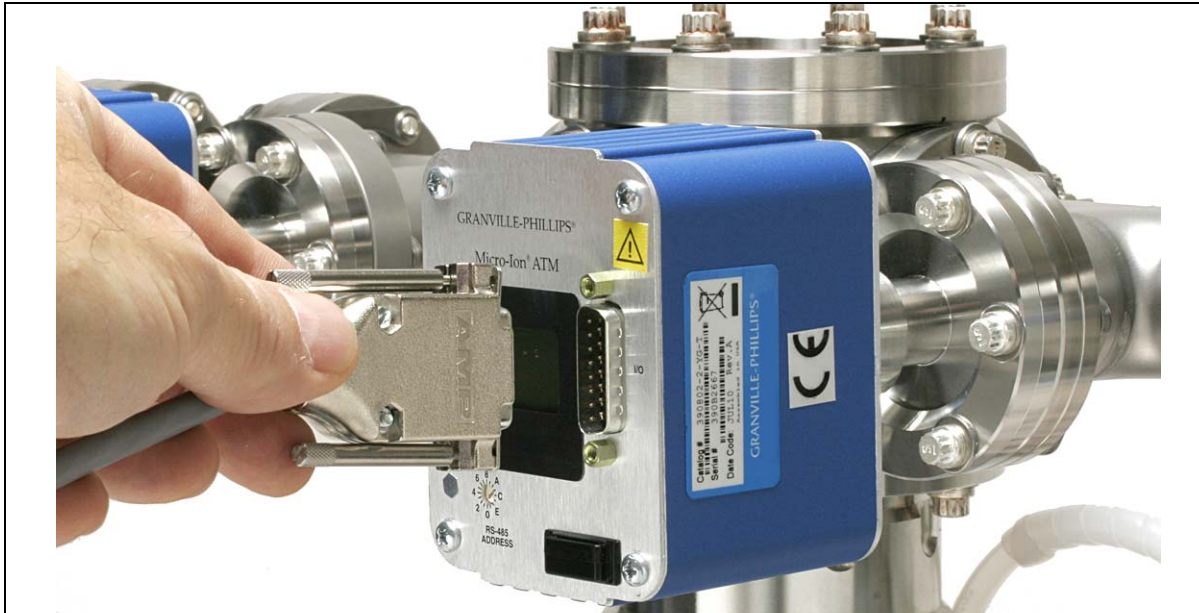
Figure 3-12 Connect the Cable to the Micro-Ion Gauge
