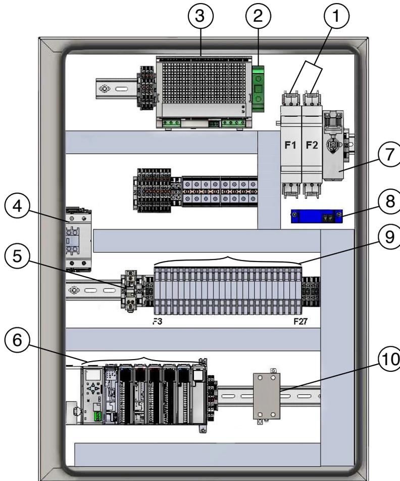
Figure 7 - Main electrical enclosure components
