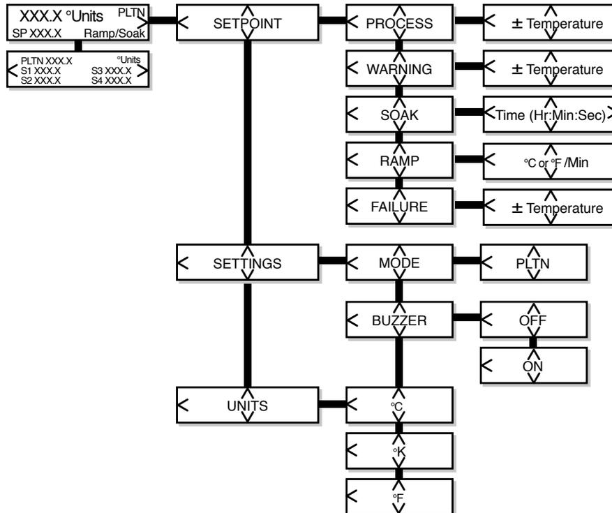
Figure 17 - Temperature controller menu flowchart
