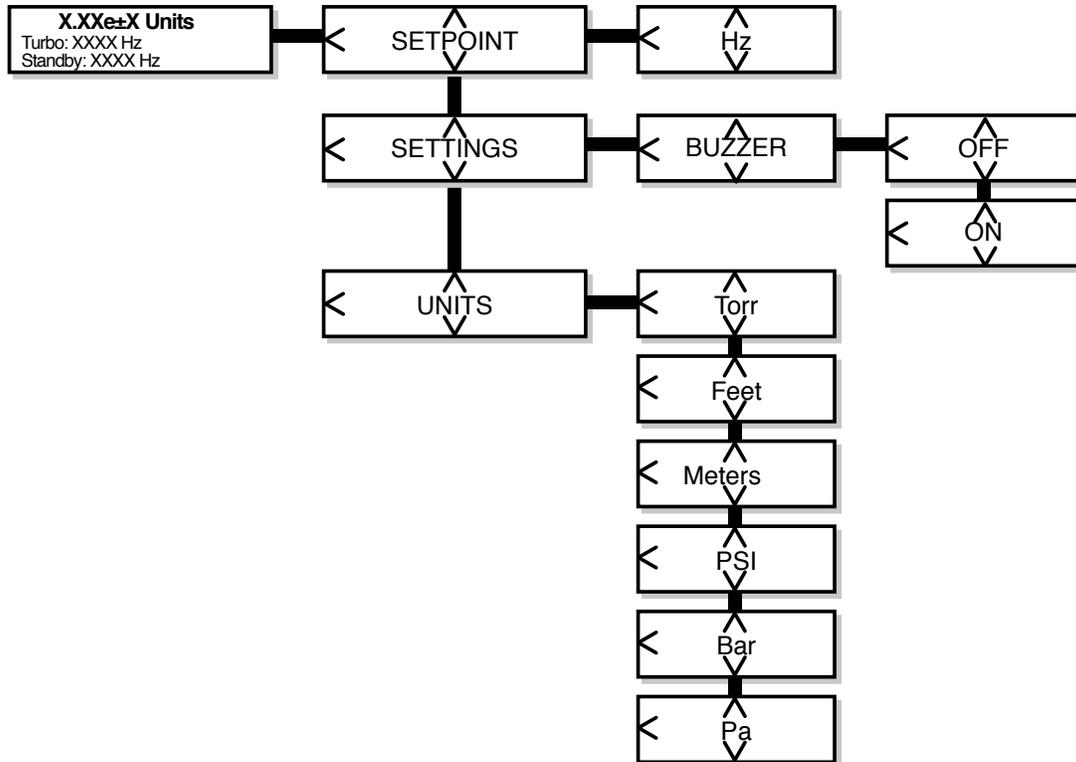
Figure 19 - Pressure gauge and turbo speed setpoint controller menu flowchart
