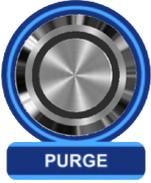
The purge function allows the user to introduce high-purity or dry gas into the chamber instead of air. Filling the chamber with purge gas instead of venting with air can be useful to keep the chamber mostly free of water when exchanging items, thereby reducing chamber pump down cycle time. Purge speed (to atmospheric pressure) is approximately 15 seconds.
