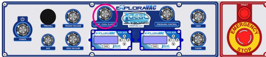
3. Set/verify the desired turbo standby speed in the Pressure gauge and turbo speed controller ([Sec. 5.11, p. 29](#)).
