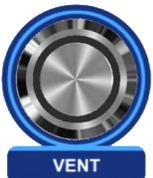
Venting is allowed only when the turbo and roughing pumps are off. If the system is in high vacuum mode, the HIGH VACUUM switch must be turned off before venting is possible. Vent speed is approximately 15 seconds.
