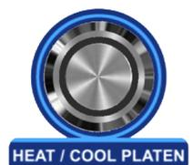
The HEAT/COOL PLATEN switch turns on the heated platen shelf. When the HEAT/COOL PLATEN switch is pressed, the switch lights green.
