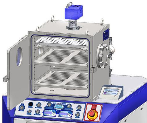
8. Press the PRESSURE CONTROL (turbo standby) switch. It illuminates green.
