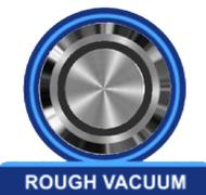
When pressed, the ROUGH VACUUM switch will light green. The nXR60i roughing pump will energize, the roughing valve will open, and the chamber will begin to pump down. The chamber will ultimately reach a pressure of about  $2 \times 10^{-2}$  Torr (20 mTorr). The XGC-820 pressure gauge and turbo speed controller will display chamber pressure.
