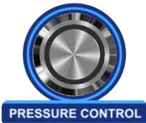
The PRESSURE CONTROL (turbo standby) switch activates the standby turbo speed programmed by the XGC-820 pressure gauge and turbo speed controller ([Sec. 5.11, p. 29](#)).
