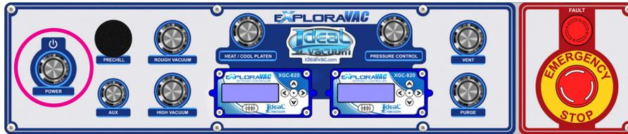
2. Verify that the HEAT/COOL PLATEN switch is off. It should be lit red.
