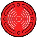
The fault light will blink and an audible buzzer will sound when a fault condition occurs. The effected subsystem switch will blink red (see Sec. 4.14, below). If the fault is because a device exceeds its parameters (i.e., an over temperature situation), the fault may self-correct. If the fault is because of equipment failure, the fault will persist. The effected device will need to be corrected before it will function.
