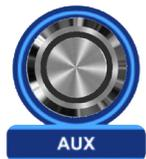
When pressed, the AUX switch will light green. The user's outboard equipment, connected to the AUX I/O relays on the digital feedthrough panel at the back of the ExploraVAC cabinet, will be powered on. ([Sec. 3.10, p. 18](#)).
