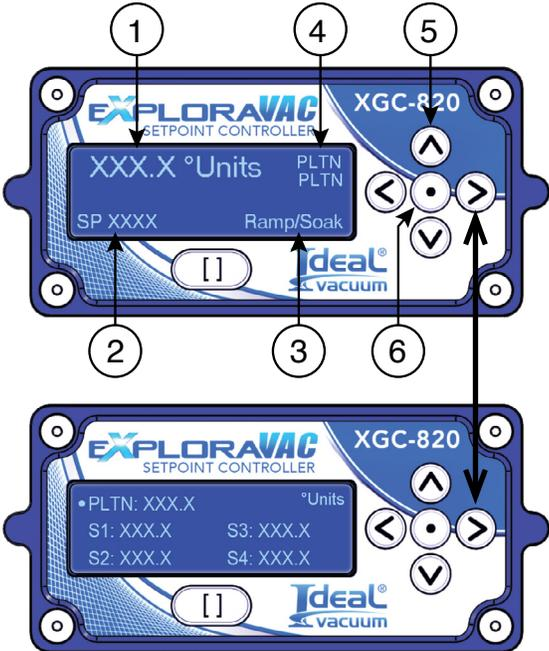
Figure 16 - Toggle between home page and thermocouple temperatures page
