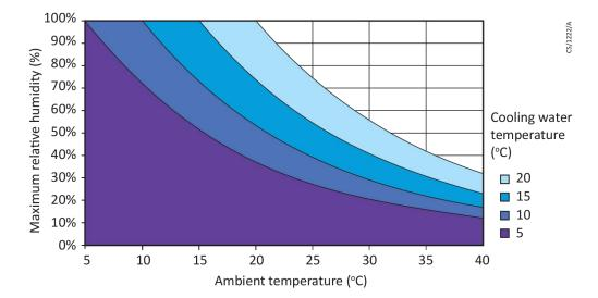
Figure 9 Maximum relative humidity to avoid condensation with water cooling
