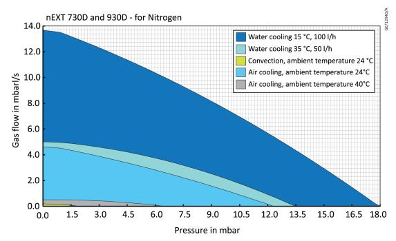
Figure 14 Cooling requirements for nitrogen for nEXT730D/930D
