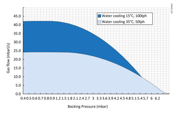
Figure 12 Cooling requirements for nitrogen for nEXT730Q/930Q
