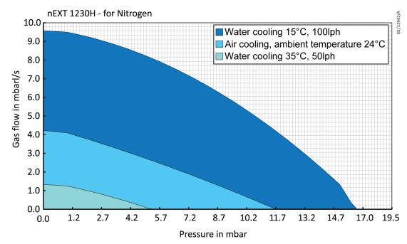
Figure 16 Cooling requirements for nitrogen for nEXT1230H
