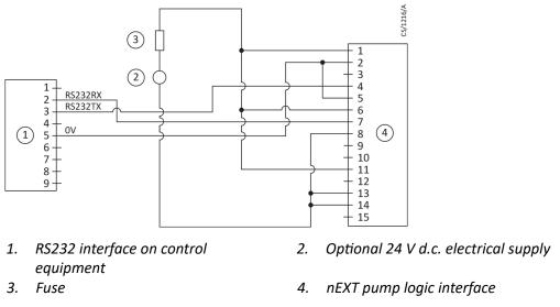
Electrical supply connection to pins 1, 6 and 11 is not required for the nEXT pump as it has a dedicated pump power supply cable. The fuse is only required if a 48 V d.c. electrical supply is connected to the logic interface cable.
