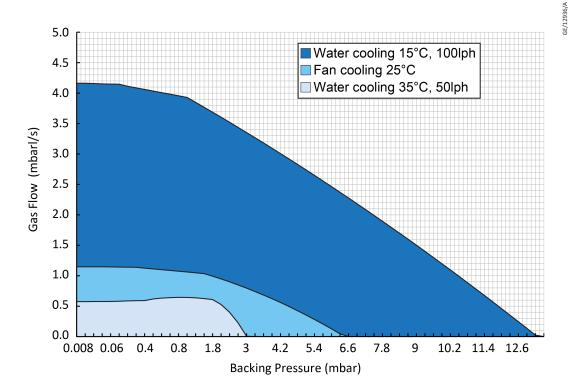
Figure 11 Cooling requirements for argon for nEXT730H
