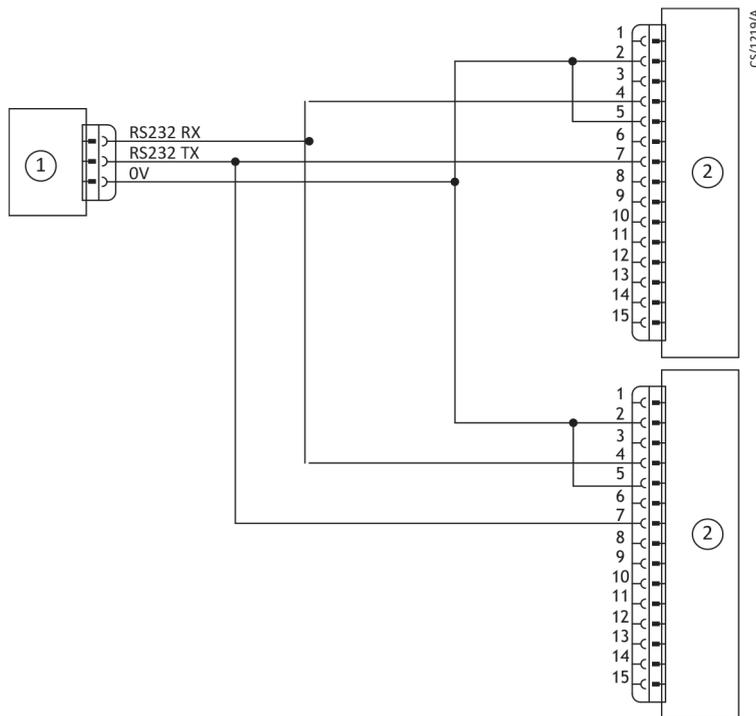
1. RS485 interface on control equipment      2. nEXT pump logic interface
