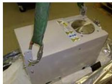
6. Wind up jacking feet until flush with bottom of chassis to expose the castors to allow the pump to be manoeuvred.
