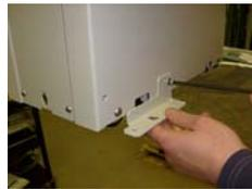
4. Reattach the brackets at the top front right and top rear left corners using 2 fixings for each bracket.
