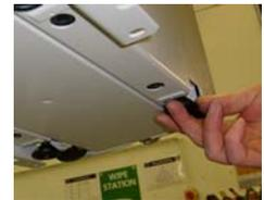
7. Lower pump to ground and remove lifting brackets. If stacking pumps then leave these brackets in place and refer to section 3.4.
