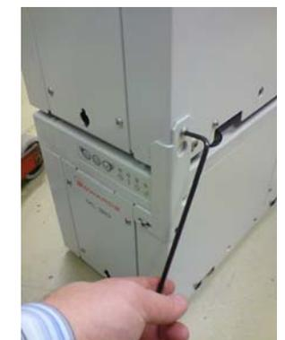
8. *Slowly* lower the *top pump* so that it rests on top of the *base pump*, and inside of the fixing brackets.
