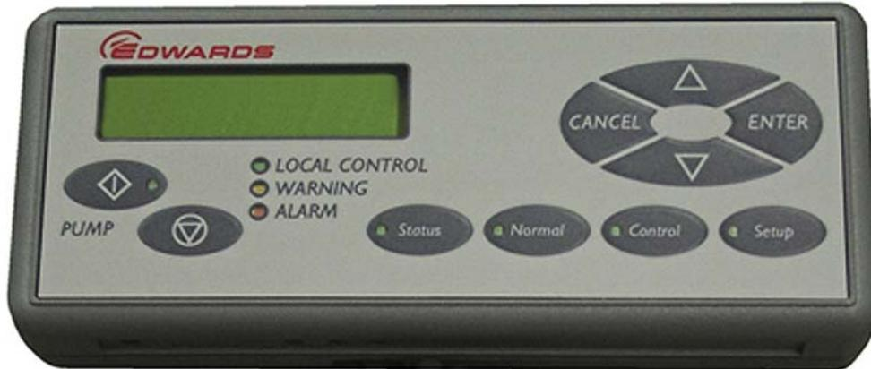
The PDT accessory provides pump on/off and status reporting. Warnings and alarms are also indicated to the user. Up to two PDTs may be fitted to the pump.
