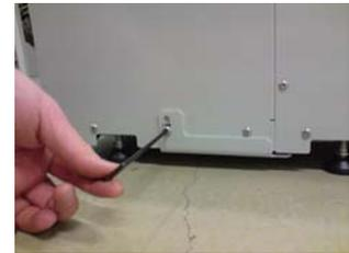
3. Reattach the brackets at the front right and rear left corners using two fixings for each bracket.
