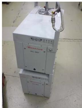
9. Attach the *top pump* to the fixing brackets using one fixing for each bracket.
