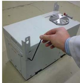
5. Attach the brackets to the *top pump* (as described above) and lift to shoulder height.
