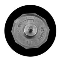
7. Lift diaphragm at the side and position carefully together with diaphragm clamping disc and diaphragm support disc in the diaphragm key.
