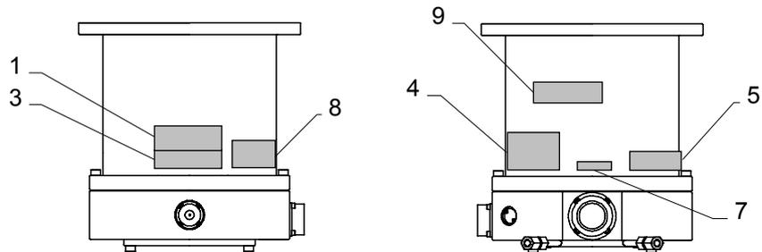
Figure 6 - Label affixing positions for the STP pump
