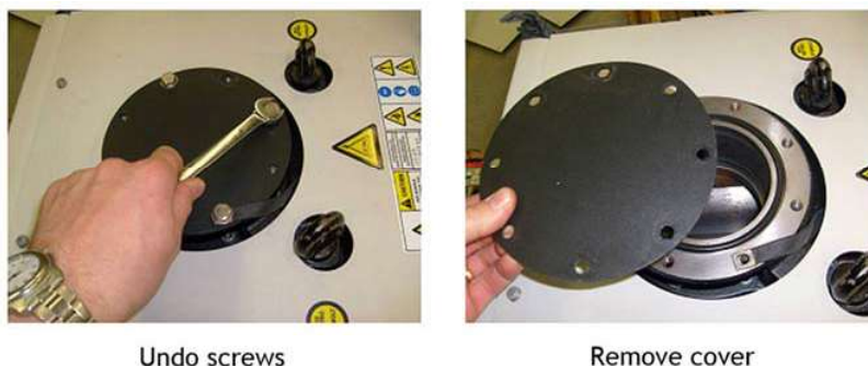
Figure 7 - Connecting the pump inlet
