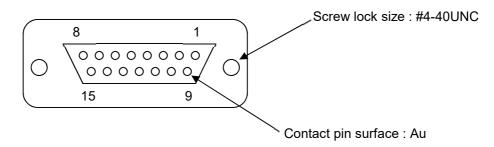
Fig 3.2 15 Pin D Sub-Miniature Female Receptacle (As seen from connecting side)
