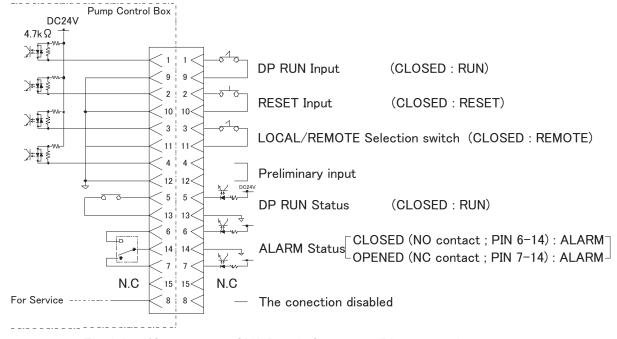
Fig.4.6 I/O connector CN2 D-sub Connector Pin connections
