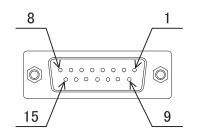
Fig.4.5 CN2 Pump-side Receptacle
