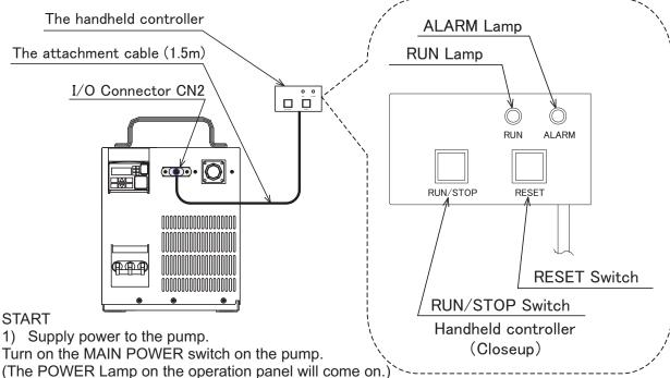
2) Press the RUN/STOP switch on the handheld controller.
