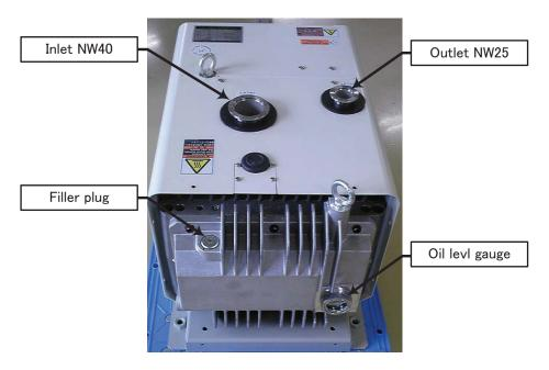
Photo 7.2 Filler plug and oil level gauge position
