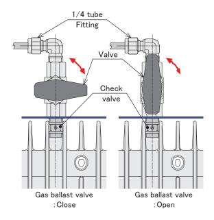
Fig. 6.1 How to open-and-close the gas ballast valve
