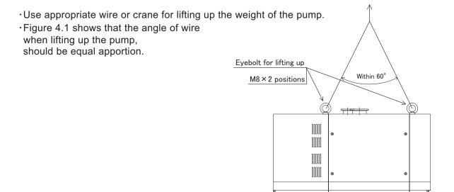
Fig. 4.1 How to Lifting up the Pump
