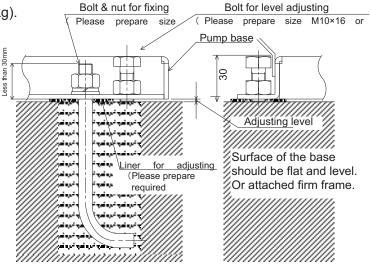
Fig.4.2 How to Fix the pump
