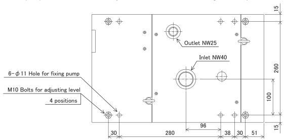
Fig.4.1 Fixing Position of the pump
