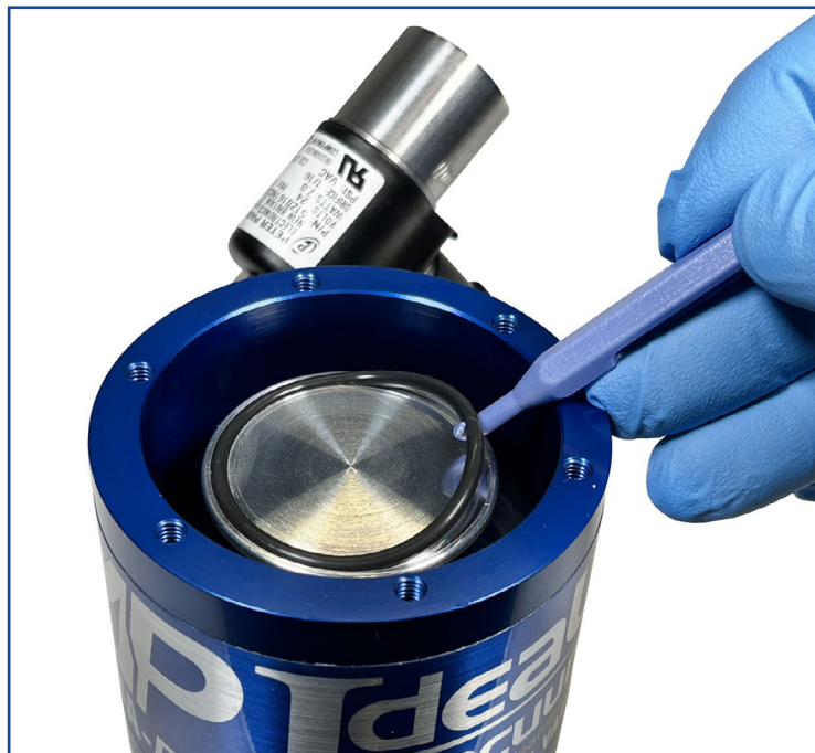
Figure 8 - Replacing the Actuator Cup O-Ring
