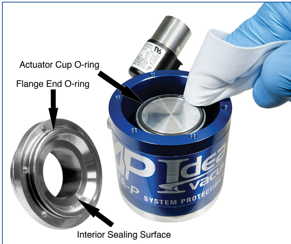
Figure 7 - Cleaning the Actuator Cup O-Ring
