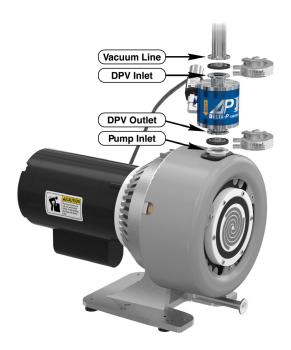
The DPV is a compact, inline unit which mounts directly on the inlet side of the mechanical pump. It is available in four standard KF flanged sizes and with three solenoid voltage options. DPV closure speed is approximately 25 ms, faster than other isolation valves.
