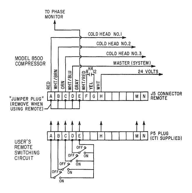
Figure F.1 Remote high-vacuum pump switching schematic
