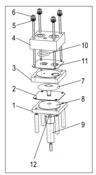
Fig. 3: Pump head (exploded drawing)
