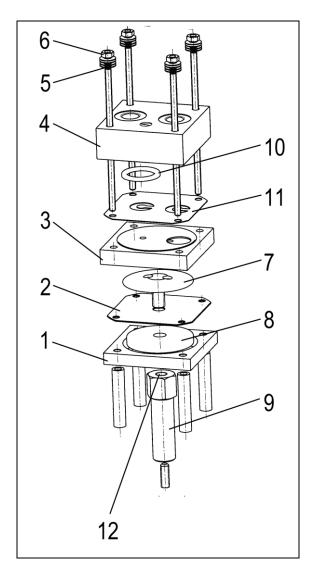
Fig. 3: Pump head (exploded drawing)
