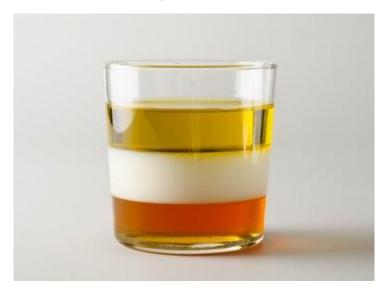
This will happen inside the vacuum pump if the two different oil types are added (hydrocarbon and fluorinated), the oil will look milky. It is important to learn that this is not harmful to the pump, both are good vacuum pump oils, they just cannot dissolve into each other.
