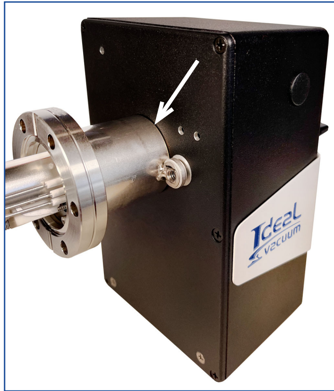
Figure 16 - Probe inserted fully into ECU
