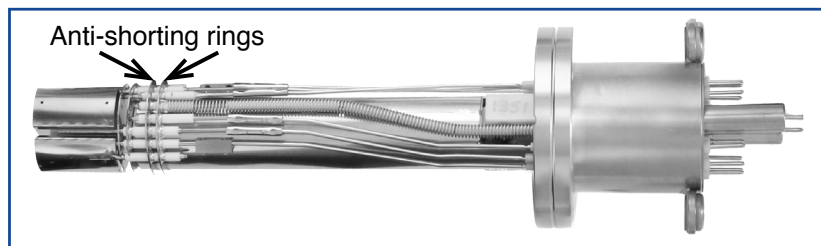
Figure 18 - Anti-shortening ring location on probe
