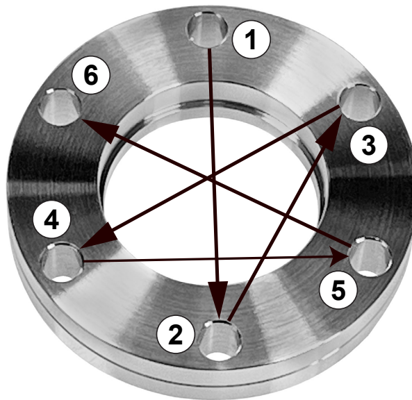
Figure 23 - Six hole tightening pattern (CF)
