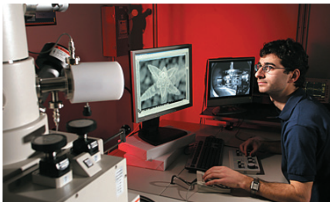
Scanning electron microscopes, like the one shown here, can "see" details as small as one nanometre – one millionth of a metre!
