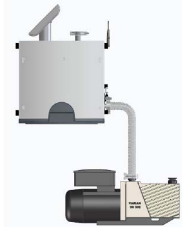
Figure 1-13 Bench Mount Leak Detector with External DS302/DS602 Wet Rotary Vane Pump, Model G8612A/GS8612D
