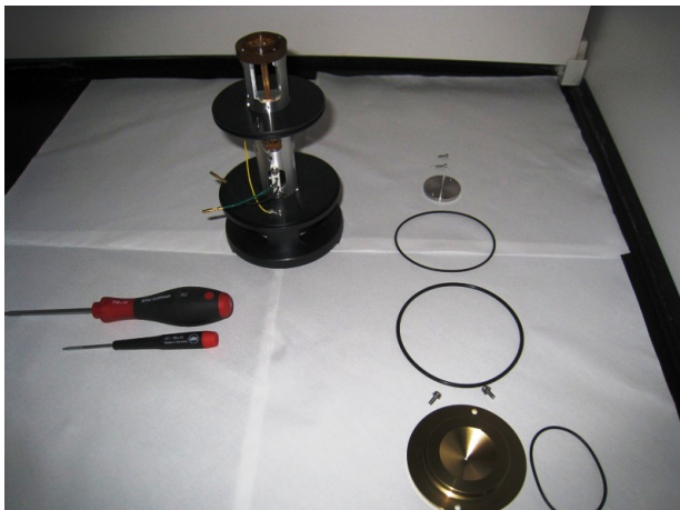
Figure 66 Skimmer and ion focus removed for cleaning
