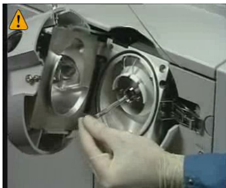
Figure 46 Reinstalling the capillary
