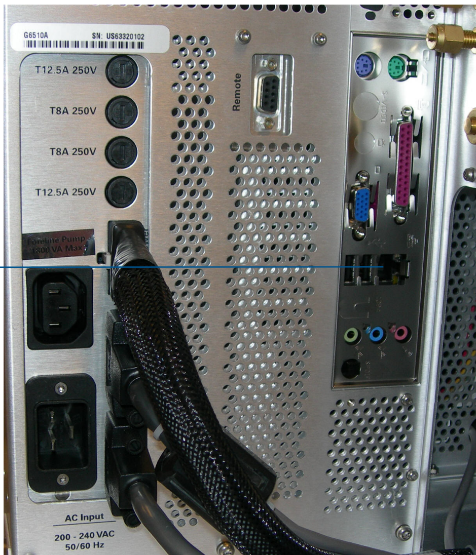
Figure 7 Gas, LAN, and power connections behind service panel for the 6400 Series and 6500 Series instruments without a pump expander box,
