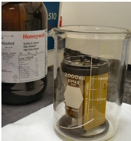
Figure 50 High pressure ion funnel in a glass beaker.
