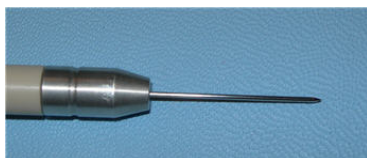
Figure 36 APCI corona needle after cleaning.
