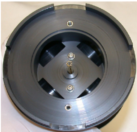
Figure 72 Octopole rods extending through skimmer spacer.
