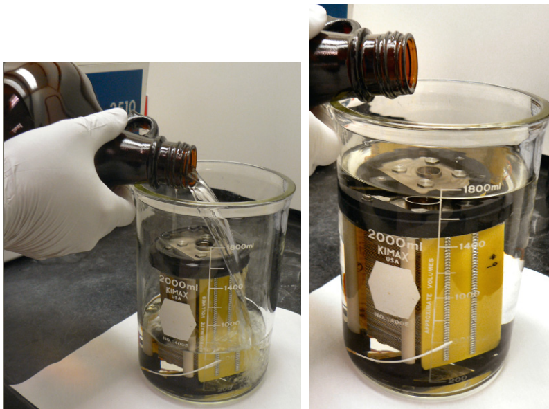
Figure 51 Pouring isopropanol into the glass beaker.
