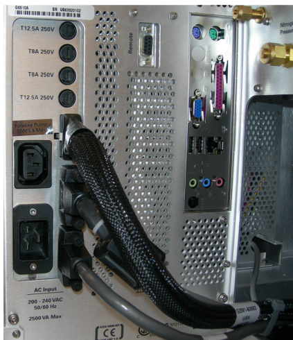
Figure 87 Disconnect the instrument power cable.
