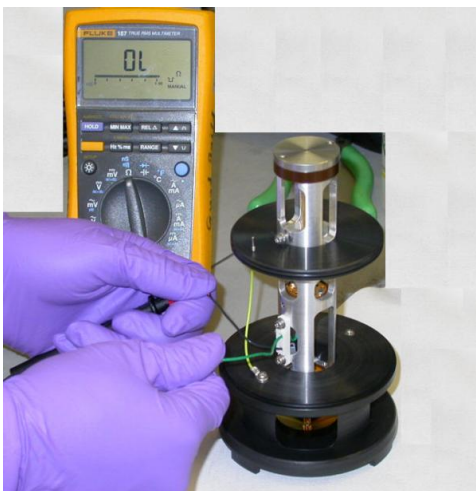
Figure 67 Testing for continuity.
