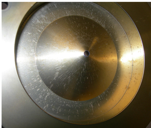
Figure 56 Sample residue on skimmer
