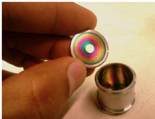
Contamination on both upper and lower sides of the plasma chamber
