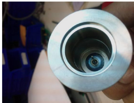
Figure 2-4 Clean Collector Chamber
