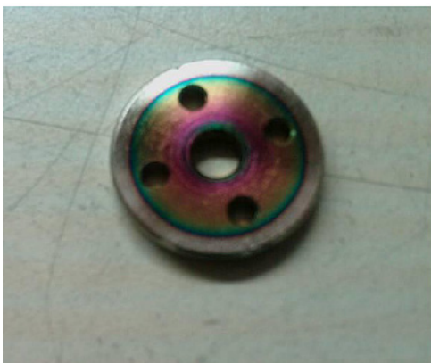
Slight contamination in the plasma region (With heavy contamination the surface is completely discolored and burnt)
