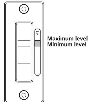
**Note:** Optimum pump performance and service life are obtained when the oil level is between the maximum level and the minimum level.
