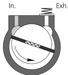
As the vane passes in front of the inlet orifice, an increasing space is formed into which the gas from the chamber to be evacuated expands. When the second vane passes, the space is closed.
