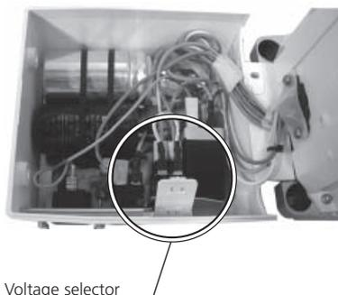
The voltage range can be read beside the motor switch: the dual frequency single-phase motor can be configured for low voltage (LV) or high voltage (HV).
