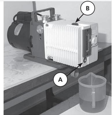
When all the oil has drained, replace the two plugs temporarily and run the pump for about 10 seconds leaving the intake open. Take care with the oil mist which may appear at the exhaust. This operation removes the oil from the functional block.
