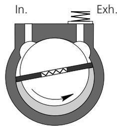
The gas trapped in the space between the two vanes is transferred to the exhaust orifice as the rotor rotates.
