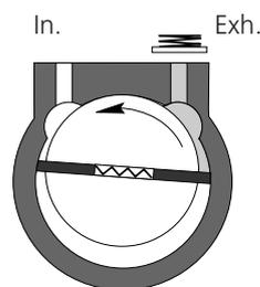
The gas is expelled into the oil casing when the pressure is sufficient to open the valve.
