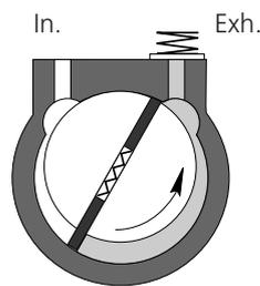
The space communicates with the exhaust, which is fitted with a valve: the gas is compressed until the safety valve is opened.
