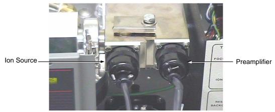
Figure 3-7 Ion Source and Preamplifier Connectors
