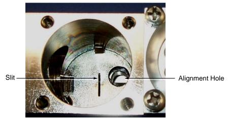
Figure 3-18 Ground Slit Plate Properly Inserted
