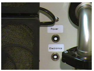
Figure 1-4 Rear Panel Circuit Breakers
