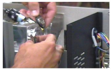
Figure 3-10 Spectrometer Tube O-ring and Centering Ring
