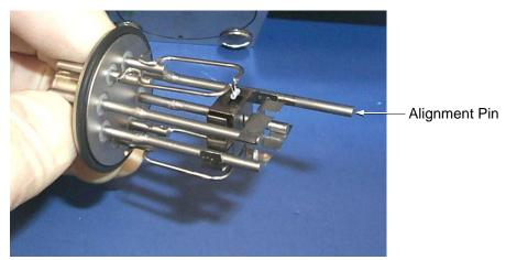
Figure 3-20 Ion Source Alignment Pin
