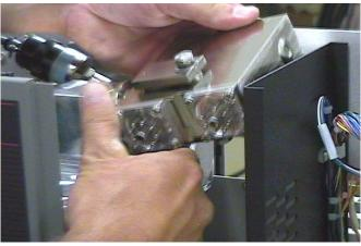
Figure 3-9 Extracting the Spectrometer Tube
