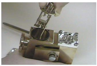
Figure 3-13 Removing the Ion Source
