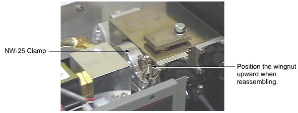
Figure 3-8 Wing Nut and Clamp
