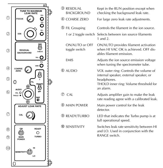
Figure 2-4 Secondary Controls and Indicators
