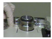
Figure 2-8 O-ring and Centering Ring on Test Port
