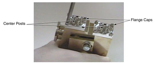
Figure 3-11 Removing Flange Cap Screws
