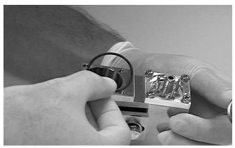
Figure 3-19 Replacing the Ion Source O-ring
