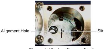
Figure 3-15 Ion Source Cavity
