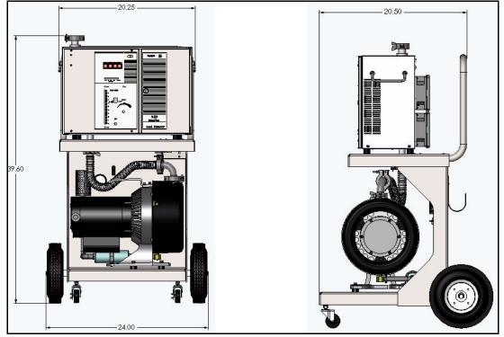
Figure 1-2 959 Dry Pump – Front and Side
