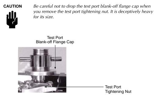
Figure 3-5 Test Port with Blank-Off Flange Cap
