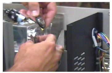
Figure 3-22 Spectrometer Tube O-ring and Centering Ring
