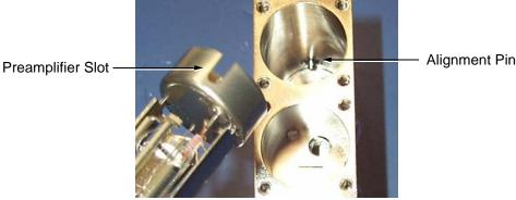
Figure 3-21 Replacing the Preamplifier
