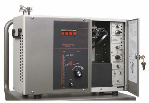
Figure 2-3 Opening the Access Panel
