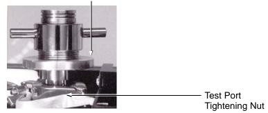
Figure 3-1 Test Port with Blank-Off Flange Cap
