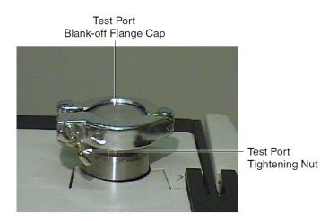
Figure 2-6 Test Port with Blank-Off Flange Cap
