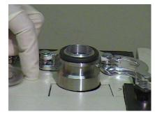
Figure 3-3 O-ring and Centering Ring on Test Port
