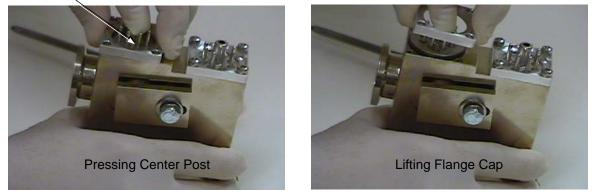
Figure 3-12 Disengaging Flange Cap
