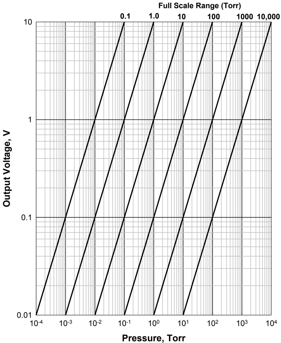
Figure 8-7 Buffered Analog Output for Capacitance Manometers
