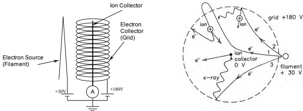
**Figure 11-5 Bayard Alpert Gauge Structure and Electron Processes**
