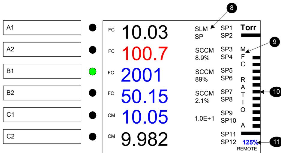
**Figure 6-1 946 LCD Front Panel Display for Pressure Measurement with either Valve Pressure Control Mode (upper) and MFC Ratio Control Mode (lower).**
