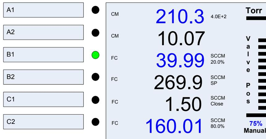
Figure 6-23 946 Display with a Pressure Control Module Installed
