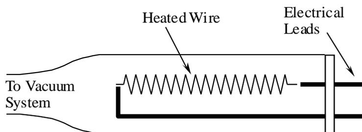
**Figure 11-7 Schematic of a Pirani Thermal Conductivity Sensor**
