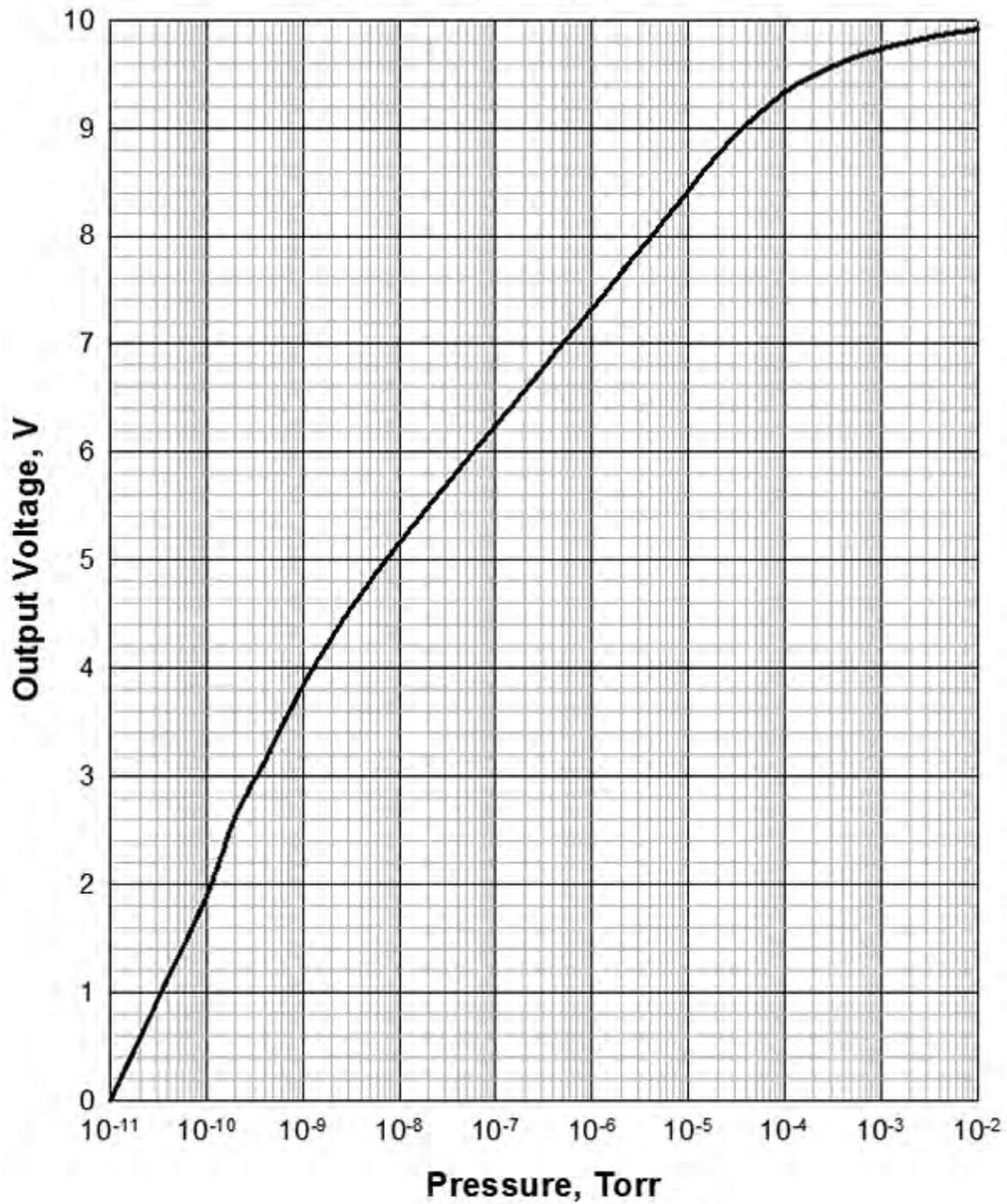
Figure 8-3 Buffered Analog Output for Cold Cathode Sensors (431/422/423) in N<sub>2</sub>
