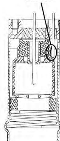
5. Slide the cathode **6**, the grid washer **5**, and the large ceramic spacer **4** into place. The grid washer **5** has a concave shape. Refer to the figures to see its installation orientation.
