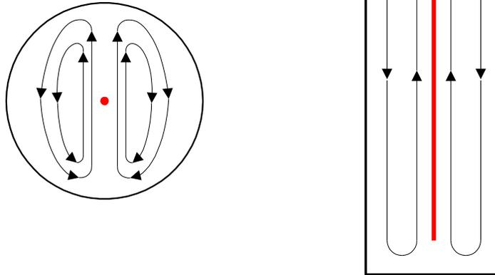
**Figure 11-8 Natural Convection Heater Transfer in Horizontal (left) and Vertical (right) Sensor Tubes.**
