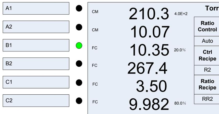
**Figure 6-21 Display with the Dialog Box for Ratio Control using Multiple MFCs**
