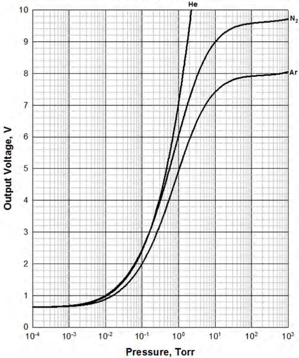
Figure 8-5 Buffered Analog Output for a 345 Pirani Sensor
