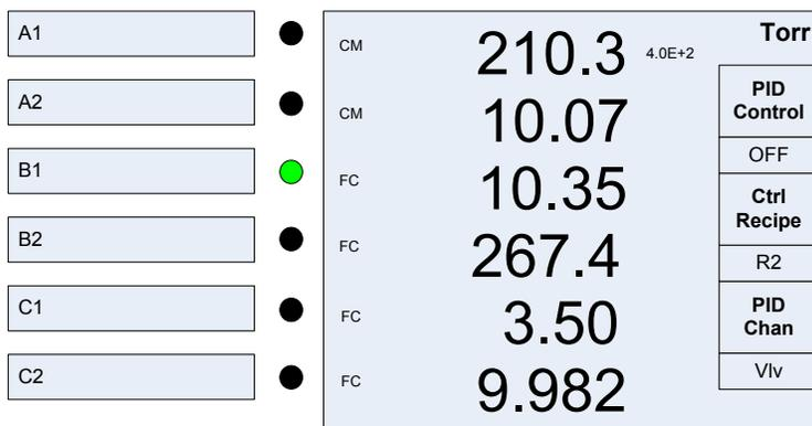
**Figure 6-27 Display with the Dialog Box for PID Control using a Valve**
