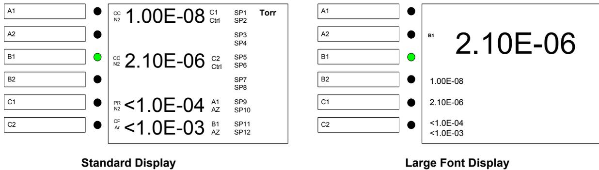
**Figure 6-2 A Comparison between Standard Display Mode and Large Font Display Mode for the 946 LCD Display During Pressure Measurement.**
