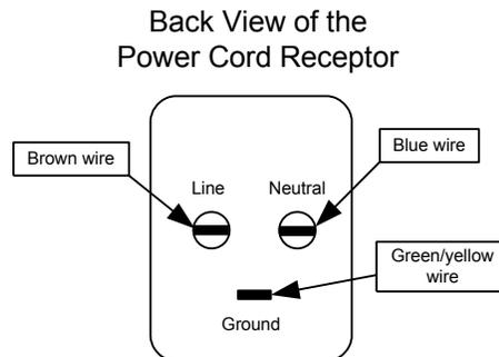
**Figure 10-2 Instruction for Connecting Wire on the Back of the Power Cord Receptor**
