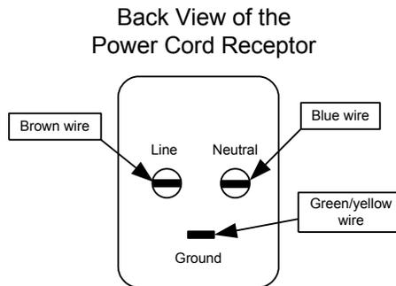
**Figure 10-2 Instruction for Connecting Wire on the Back of the Power Cord Receptor**
