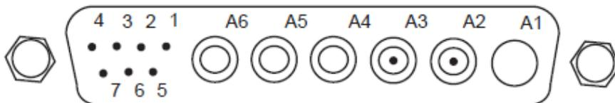
Figure 7-1 Connector on the Back of the HC Module
