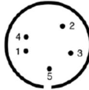
Figure 11-9 Series 275 Convector Sensor Base Pinout
