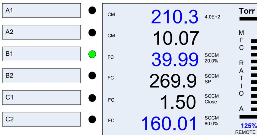
**Figure 6-22 Display during Ratio Control using Multiple MFCs**
