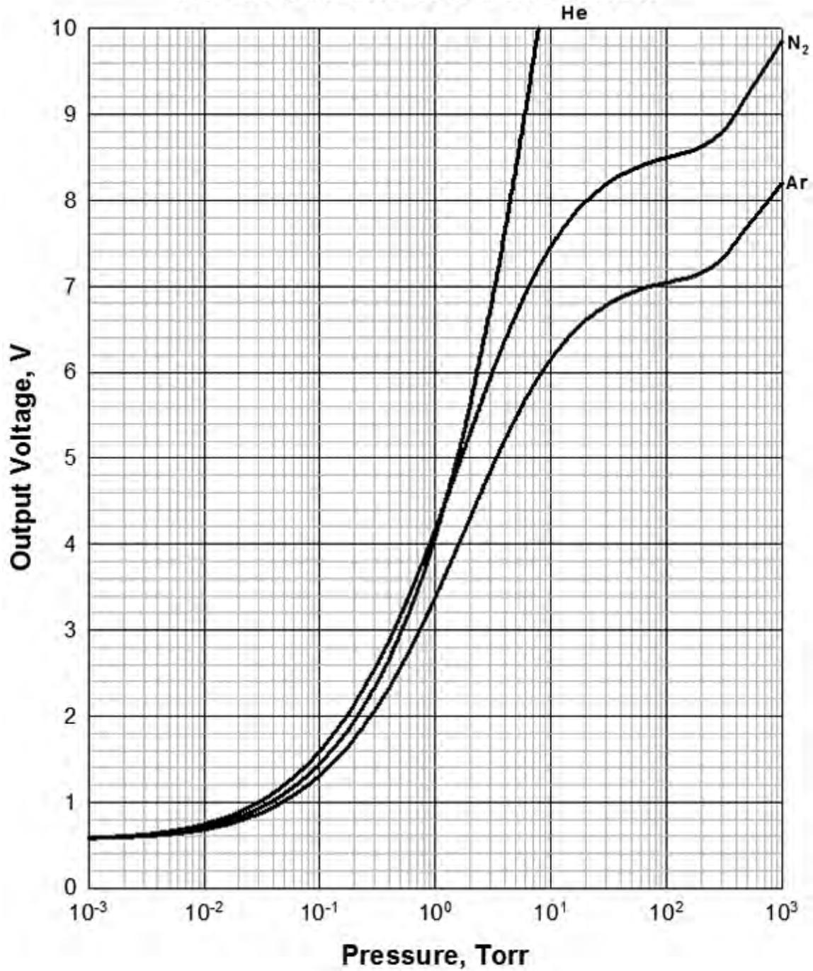
Figure 8-6 Buffered Analog Output for the 317 Convection Pirani Sensor
