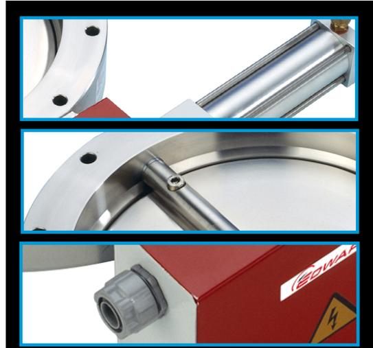
The QSB quarter swing valves are compact, quick acting, high conductance isolation valves. The QSB valves have a polished, stainless steel, ISO flanged body with fluoroelastomer 'O' ring sealed valve plate and shaft. The valve plate 'O' ring groove is vented to help maintain a stable high vacuum. The valve shaft 'O' rings and bearings are lubricated with Fomblin® grease to prevent gas bursts from behind the shaft seals.
