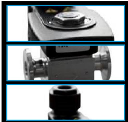
The IPVA10EK is a solenoid operated valve designed for automatic admittance of air or vent gas into a vacuum system. The valve has two ports with NW flanges. One of the valve ports is connected to the vacuum system, the other port can be left open to atmosphere or connected to a vent gas supply. The vacuum system is isolated from atmosphere (or the vent gas supply) by a fluoroelastomer pad on the base of the valve plunger, which seals against the body of the valve.
