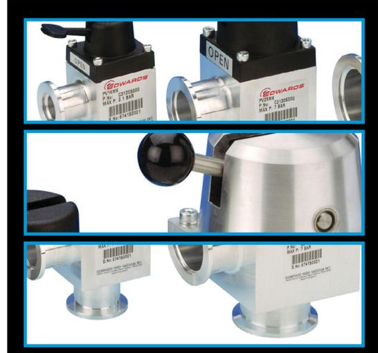
The PVMK is a quick acting, bellows sealed, right-angled lever operated valve and is available with either an aluminium or stainless steel body. The lever, connected to a self lubricating plastic cam-piston, actuates the valve stem and valve plate through PTFE bearings. The valve plate 'O' ring groove is vented to prevent gas bursts. The valves are designed to operate down to  $10^{-9}$  mbar/  $8 \times 10^{-10}$  Torr and up to a pressure of 2100 mbar/1575 Torr (30 psi).
