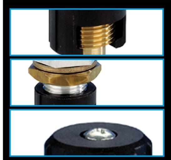
The AV5A is manufactured in aluminium alloy. It has a control knob attached to a screw-actuated plunger: turn the control knob clockwise to close the valve. A nitrile 'O' ring seals the plunger to the valve body.
