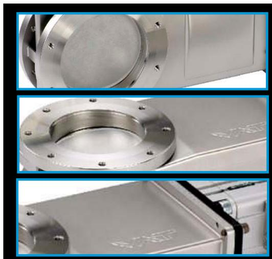
Edwards BGV gate valves are bellows sealed stainless steel gate valves for use in applications which require high leak tightness and a minimum of hydrocarbons in the vacuum system. Although principally designed for the isolation of pumps in the semiconductor fab basement, BGV gate valves are also ideal in other applications where a 1 bar differential at opening is desirable.
