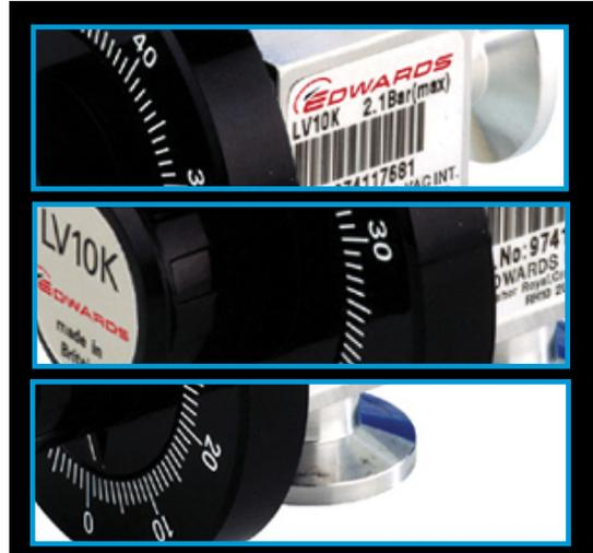
The LV10K needle valve provides fine control of gas bleed into a vacuum chamber or a regulated leak to control pressure in a vacuum system and is suitable for gas admission down to  $10^{-5}$  mbar /  $8 \times 10^{-6}$  Torr. Suitable for pipeline or panel mounting.
