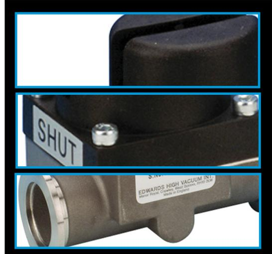
The IPVMK is a quick acting, bellows sealed, right-angled lever operated valve and is available with either an Aluminium or stainless steel body. The lever, connected to a self lubricating plastic cam-piston, actuates the valve stem and valve plate through PTFE bearings. The valve plate O-ring groove is vented to prevent gas bursts. The valves are designed to operate down to  $10^{-9}$  mbar /  $8 \times 10^{-10}$  Torr and up to a pressure of 2100 mbar/1575 Torr (30 psi).
