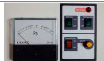
Pirani Vacuum Gauge and Control Panel
