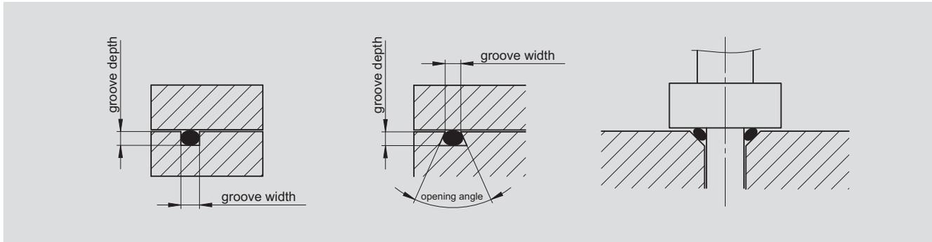
Figure 3.6: O-ring seals in rectangular groove, trapezoidal-groove and in an angular position
