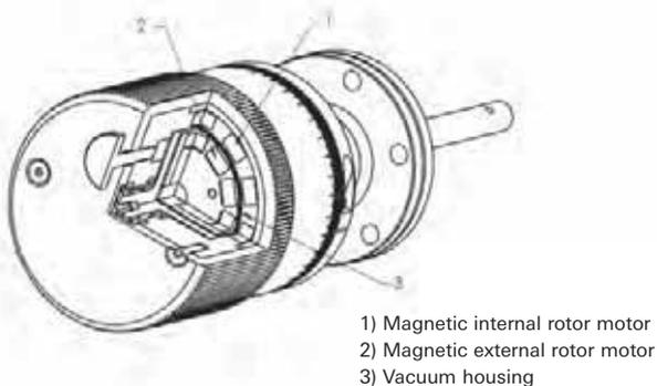
Figure 3.26: Magnetically coupled UHV rotary feedthrough
