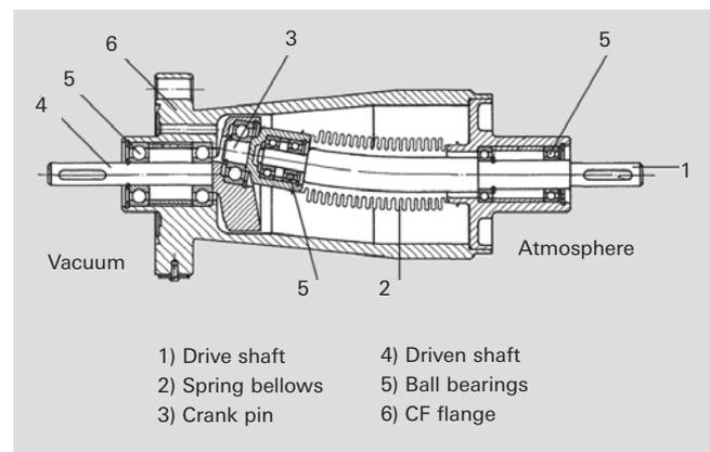
Figure 3.25: Bellows-sealed UHV rotary feedthrough (cattail principle)
