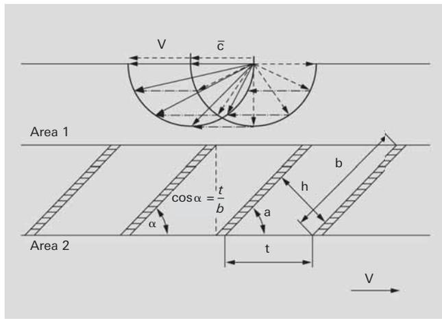
Figure 4.22: Operating principle of the turbomolecular pump
