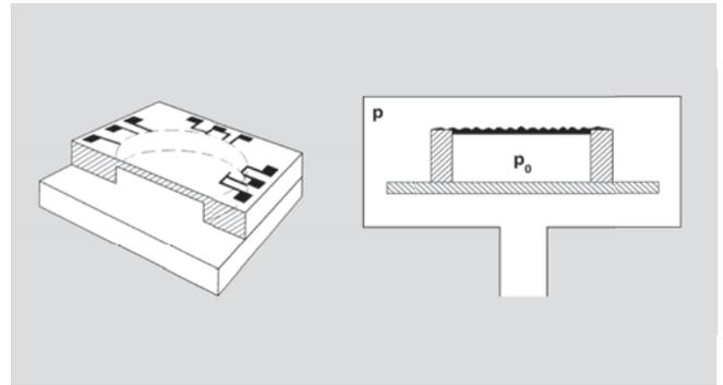
Figure 5.1: Design of a diaphragm vacuum gauge
