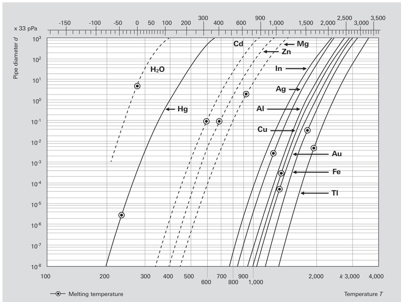
Figure 1.9: Vapor pressure curves of various substances [14]
