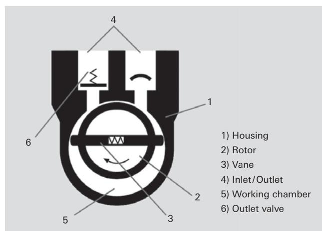
**Figure 4.2:** Operating principle of a rotary vane pump
