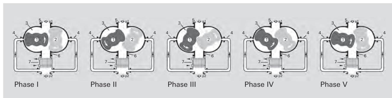
Figure 4.17: Operating principle of a gas cooled Roots pump
