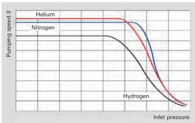
**Figure 4.25:** Pumping speed as a function of inlet pressure
