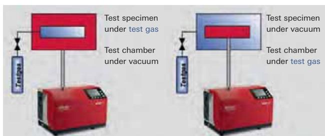
Figure 7.7: Integral leak detection with the vacuum method
