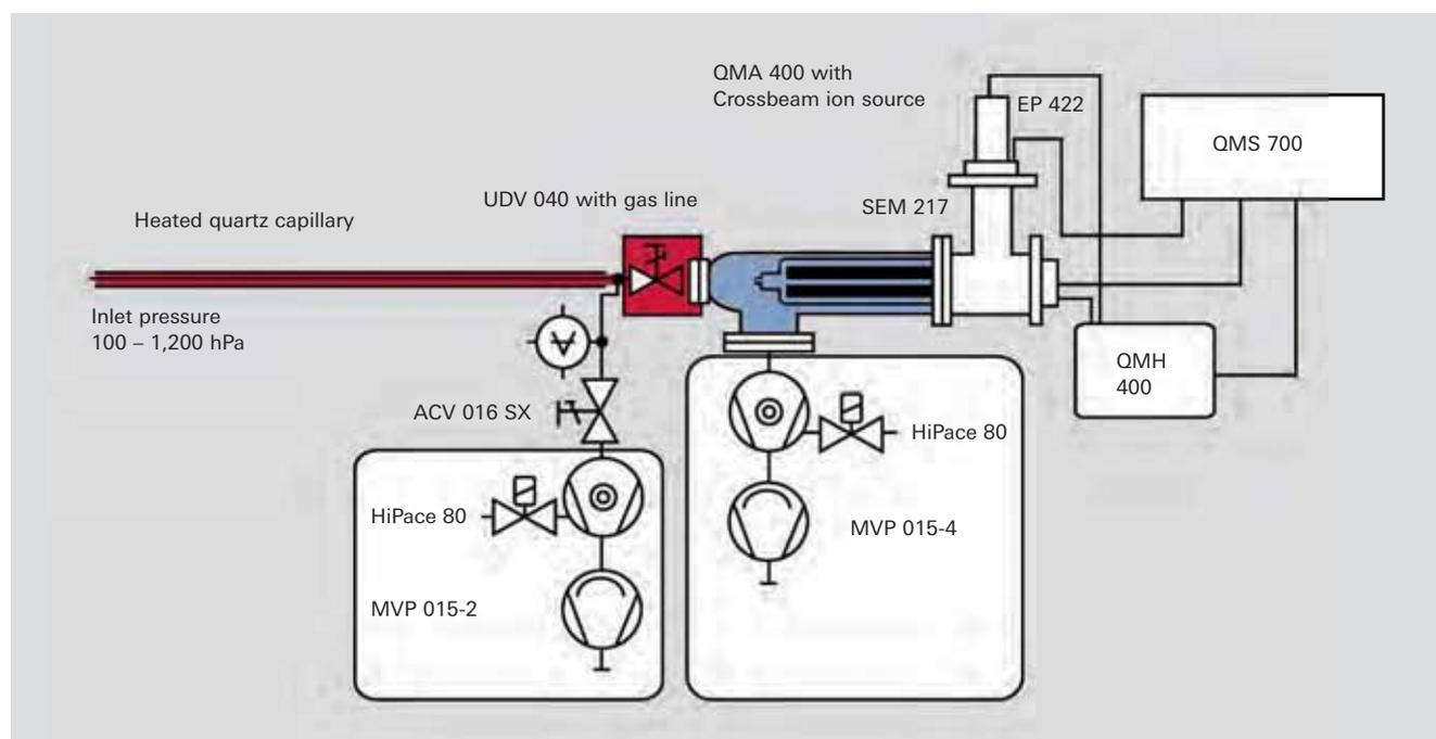
Figure 6.18: QMS with gas inlet system and crossbeam ion source
