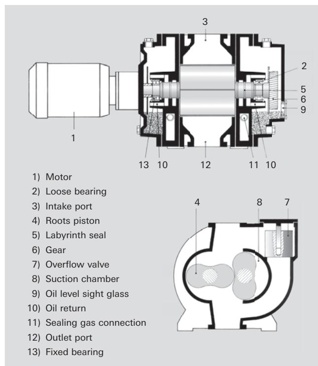
Figure 4.16: Operating principle of a Roots pump
