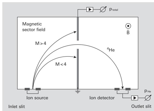
**Figure 6.3:** Operating principle of the 180° sector mass spectrometer
