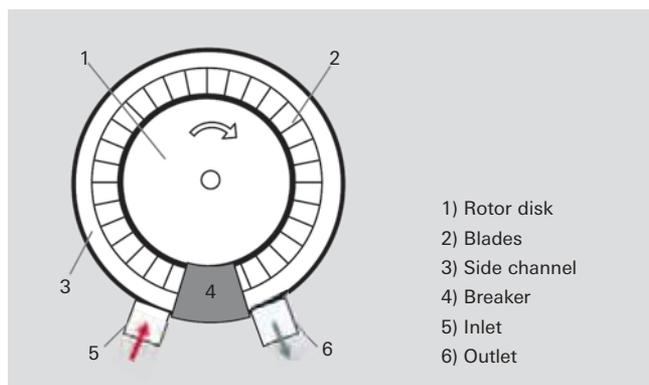
Figure 4.20: Operating principle of a side channel vacuum pump
