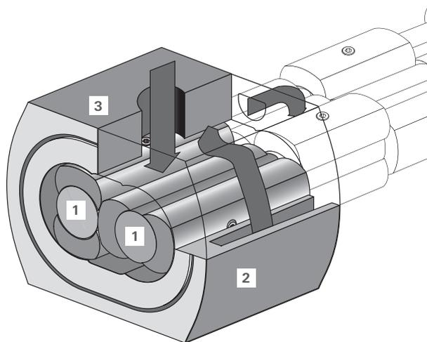
**Figure 4.11:** Operating principle of a multi-stage Roots pump, process pump
