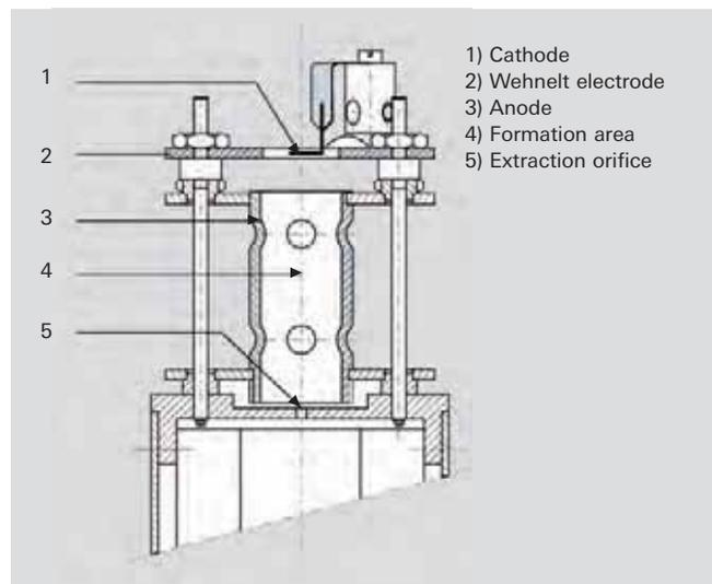
Figure 6.6: Section through an axial ion source.
