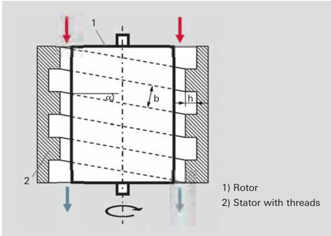
Figure 4.26: Operating principle of a Holweck stage
