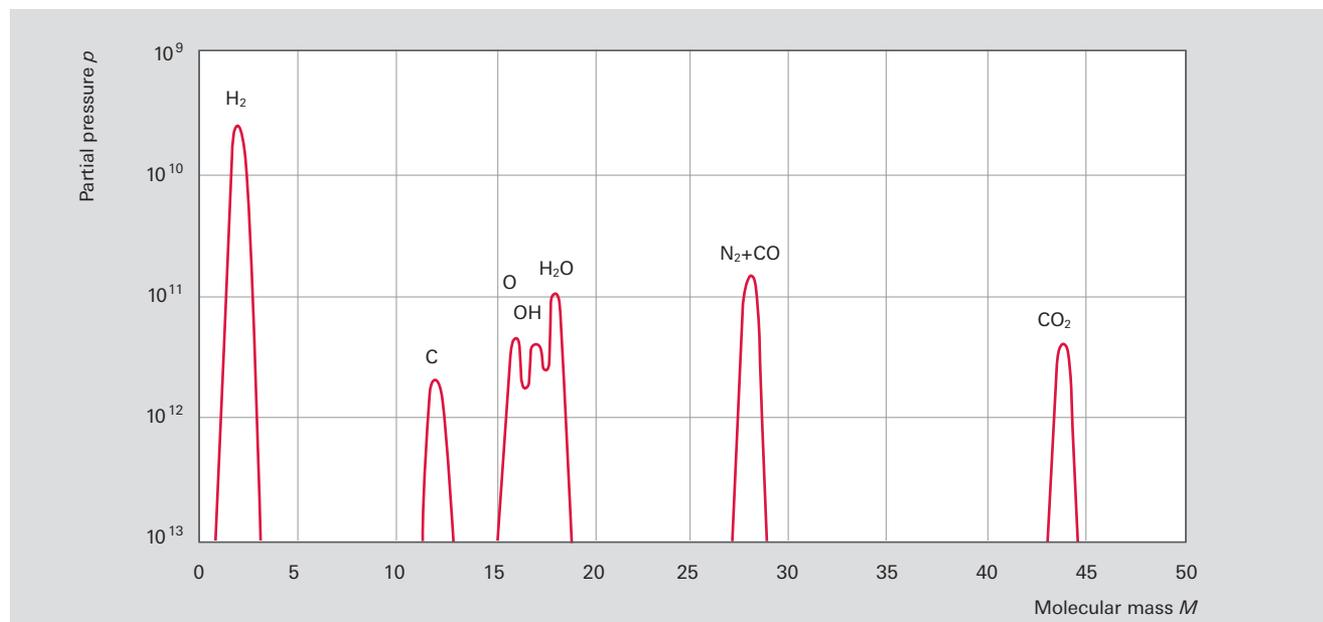
Figure 4.28: Typical UHV residual gas spectrum (turbopump)
