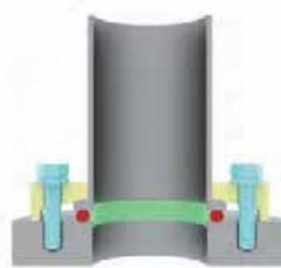
Figure 3.8: ISO-KF flange mounted on base plate with centering ring and claw clamps
