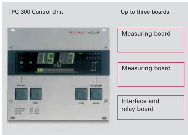
Figure 5.11: TPG 300 control unit for ModulLine sensors
