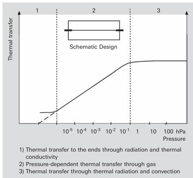
Figure 5.3: Operating principle of the Pirani vacuum gauge.
