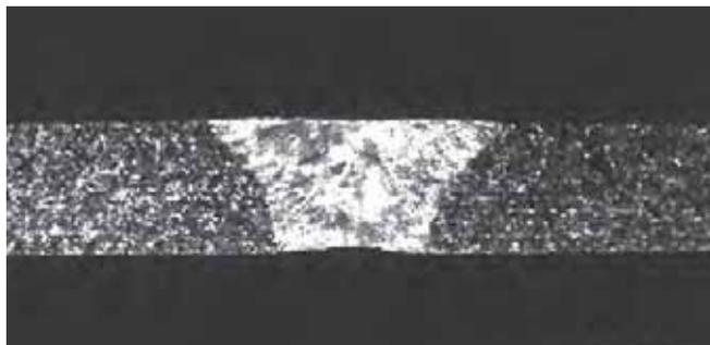
Figure 3.5: Cross section image of WIG orbital weld
