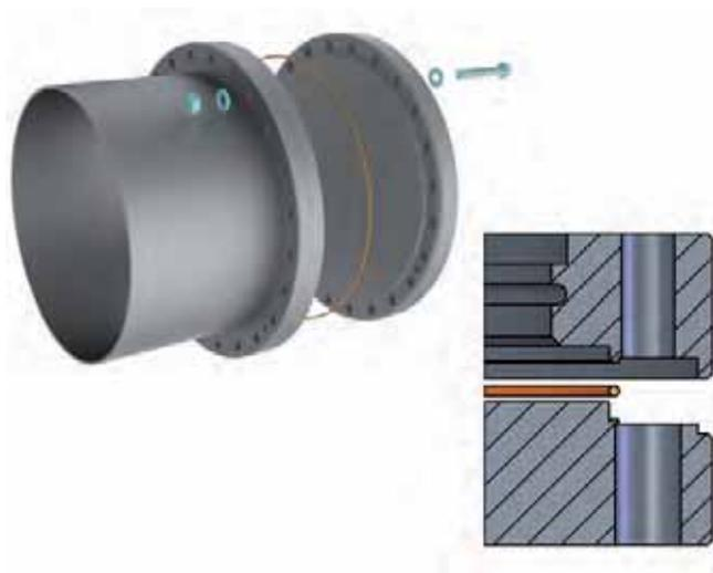
Figure 3.16: COF connection with copper wire seal and screws
