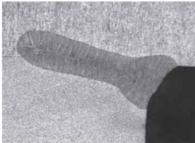
Figure 3.4: Cross section image of a laser weld
