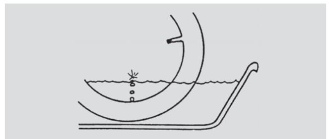
Figure 7.1: Bubble leak test on a bicycle tube
