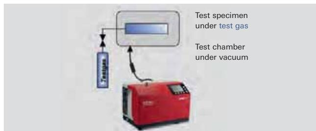
Figure 7.8: Integral leak detection of enclosed objects with the sniffer method
