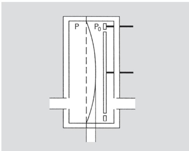
Figure 5.2: Design of a capacitive diaphragm vacuum gauge
