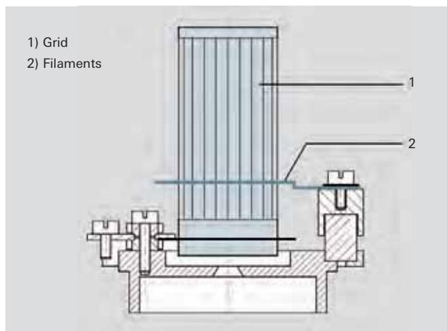
**Figure 6.9:** Grid ion source
