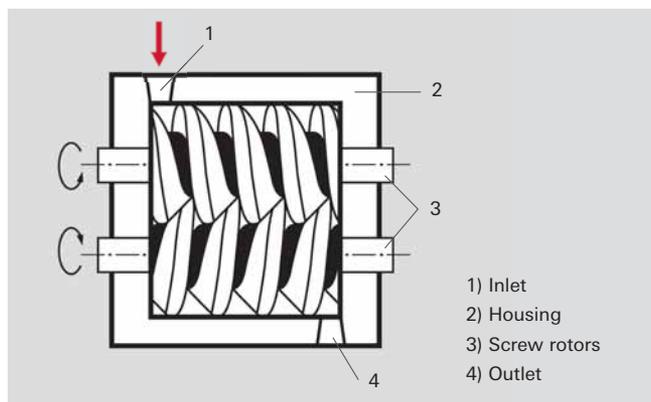
Figure 4.6: Operating principle of a screw pump
