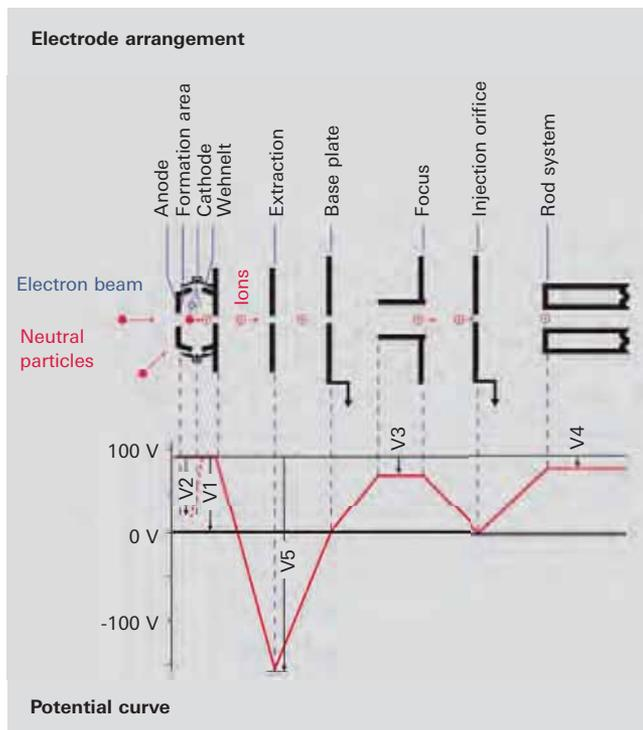
Figure 6.20: Potential curve in an electrically biased ion source
