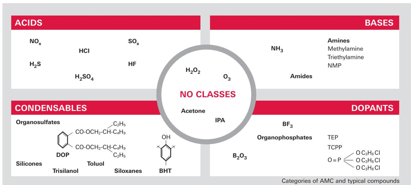
Figure 8.4: Classification of airborne molecular contamination AMC
