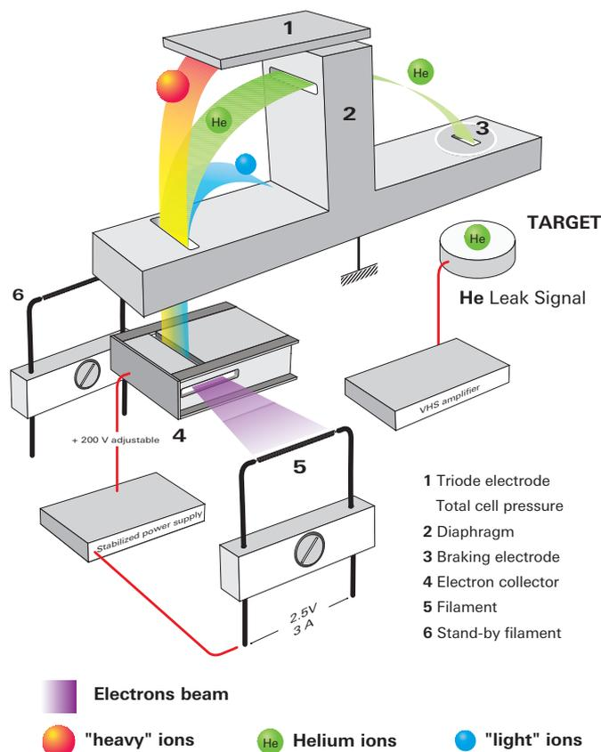
Figure 7.2: Working principle of a sector mass spectrometer
