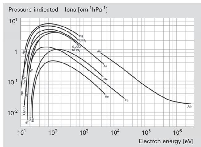
Figure 6.7: Ionization as a function of electron energy
