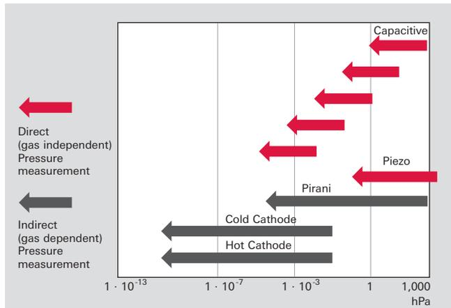
Figure 5.8: Pressure measurement ranges and measurement principles
