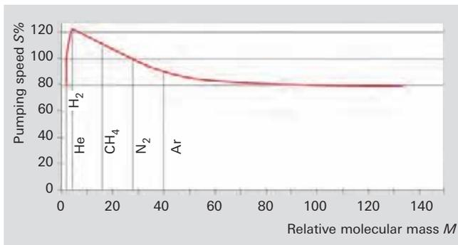
**Figure 4.24:** Pumping speed as a function of relative molecular mass
