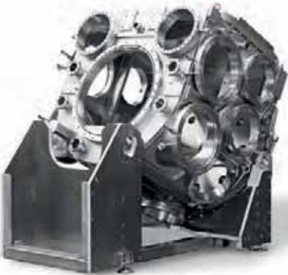
**Figure 3.17:** EUV source chamber with cooling profiles and water-cooled flanges
