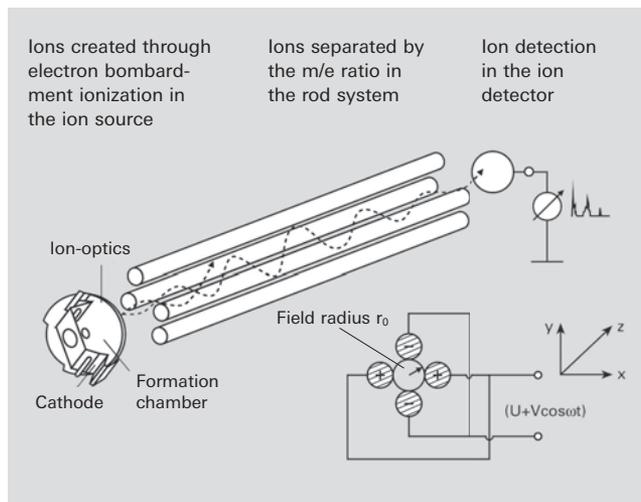
Figure 6-5: Operating principle of a quadrupole mass spectrometer
