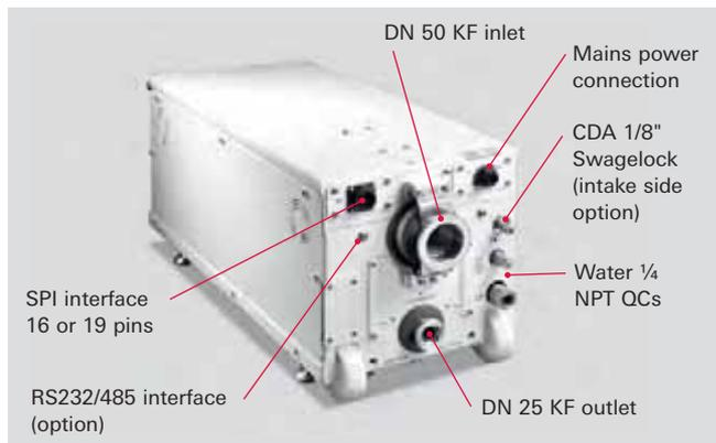
Figure 4.13: A 100 L rear side with connections
