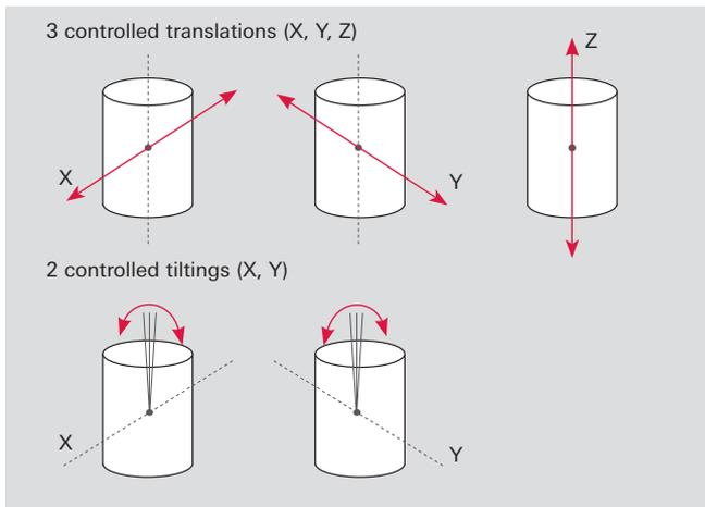
Figure 4.21: Degrees of freedom of a turbo-rotor
