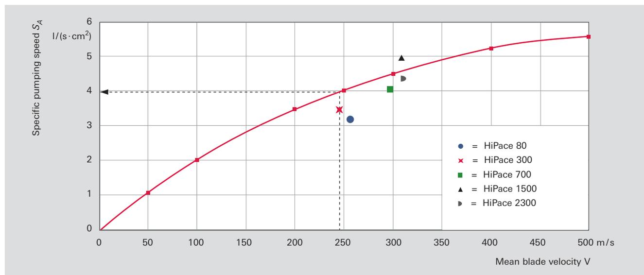
**Figure 4.23:** Specific turbopump pumping speeds
