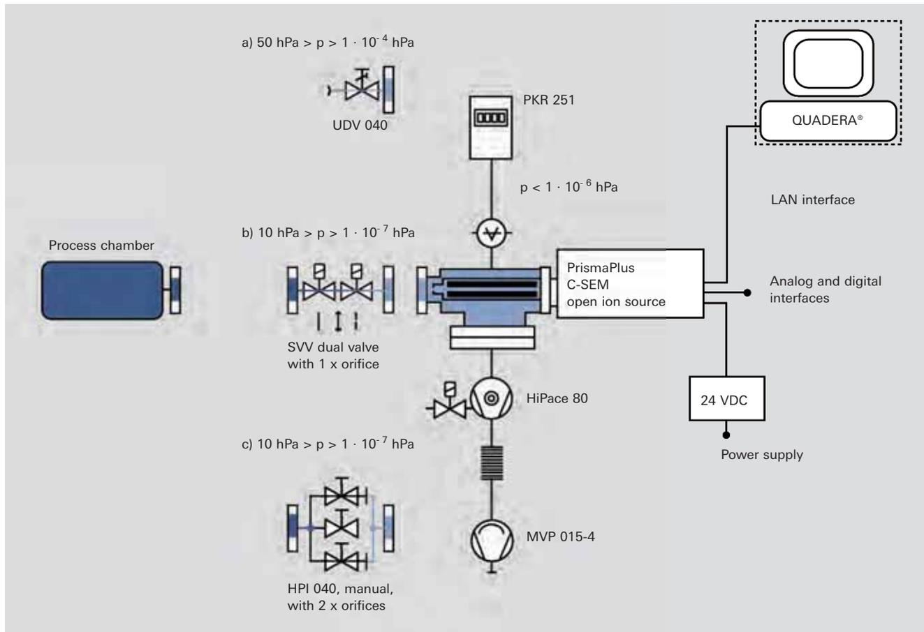
Figure 6.19: Differentially pumped QMS with various gas inlets
