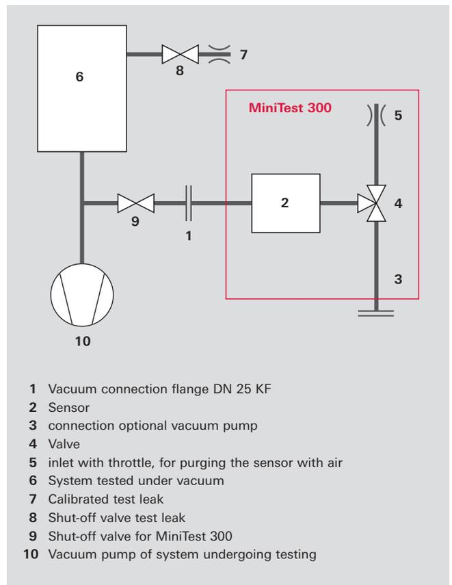
Figure 7.5: Vacuum diagram of the MiniTest quartz window leak detector on a system
