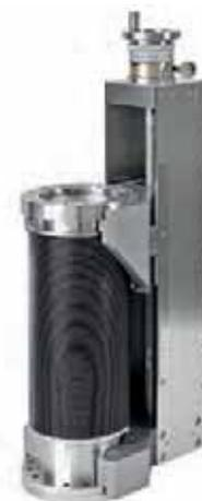
Figure 3.28: Z-axis precision manipulator
