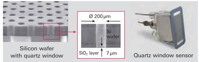
Figure 7.4: Operating principle of quartz window sensor
