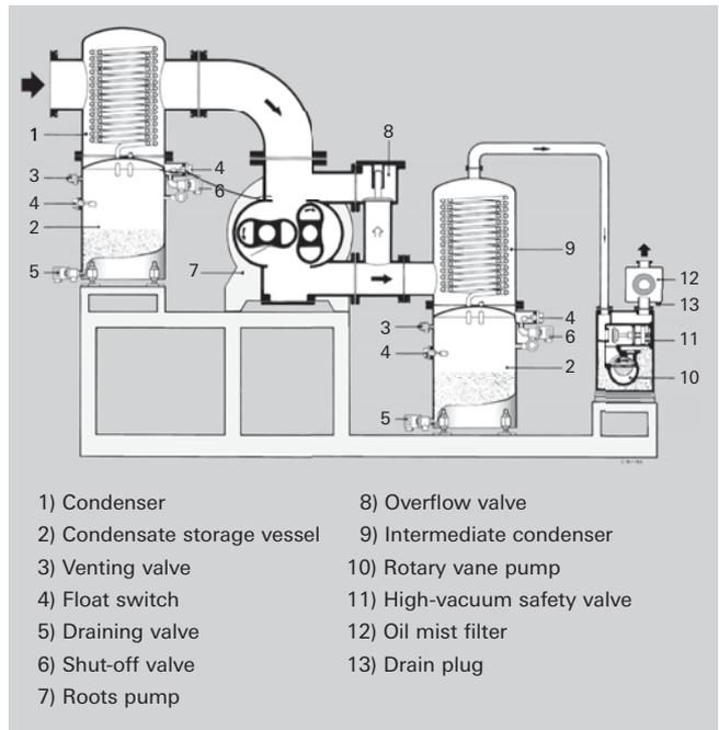
**Figure 2.4:** Roots pumping station for vapor condensation
