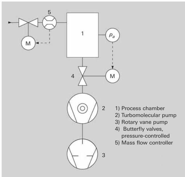
Figure 2.8: Vacuum system with pressure and throughput regulation
