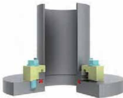
**Figure 3.11:** ISO-K flange mounted on base plate with O-ring nut and claw clamps for base plate with sealing groove
