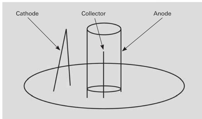
Figure 5.7: Design of a Bayard-Alpert vacuum gauge
