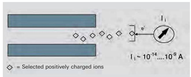
Figure 6.15: Operating principle of a Faraday Cup
