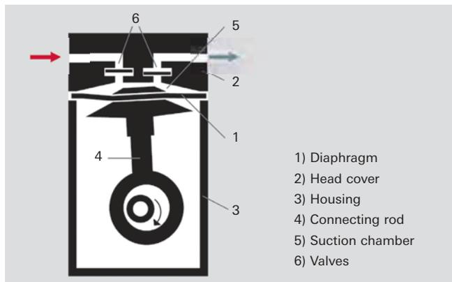
Figure 4.5: Operating principle of a diaphragm vacuum pump
