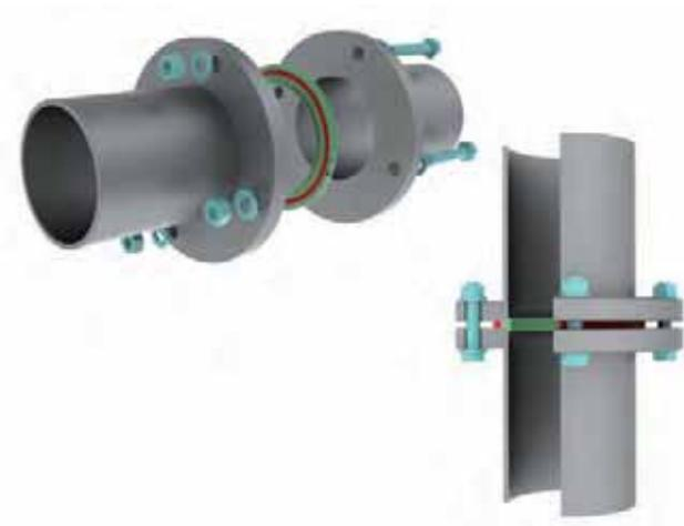
**Figure 3.13:** ISO-F connection with centering ring and screws
