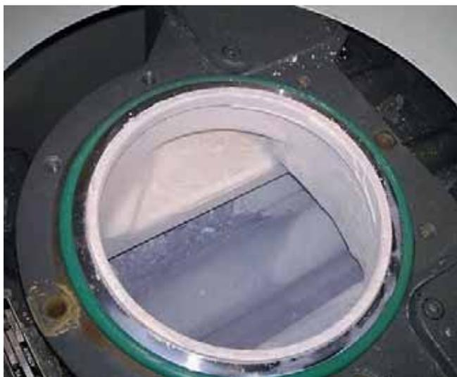
**Figure 4.10:** Condensation of ammonium hexafluorosilicate  $(\text{NH}_4)_2\text{SiF}_6$  in a Roots pump operated at too low a temperature
