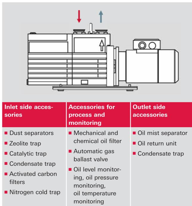
Figure 4.4: Accessories for rotary vane pumps
