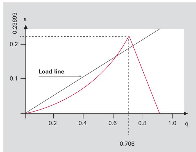
**Figure 6.6:** Stability diagram of a quadrupole filter
