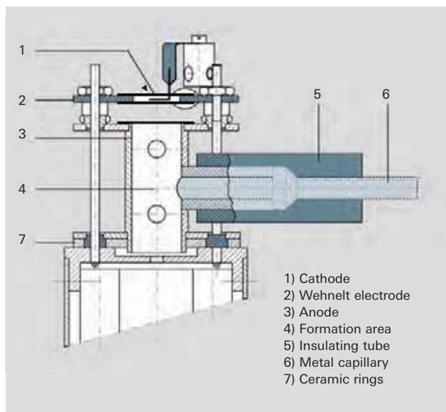
Figure 6.12: Gas-tight axial ion source
