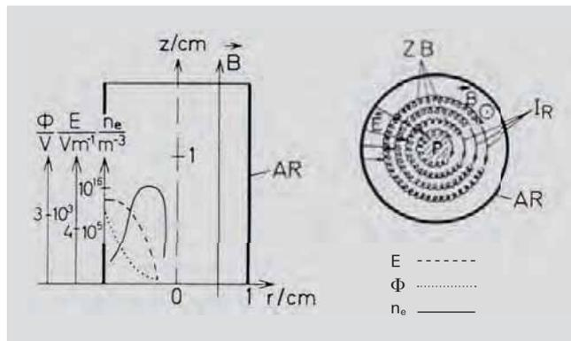
Figure 5.6: Operating principle of an inverted magnetron
