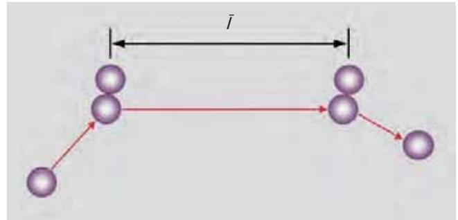
**Figure 1.4:** Mean free path between two collisions
