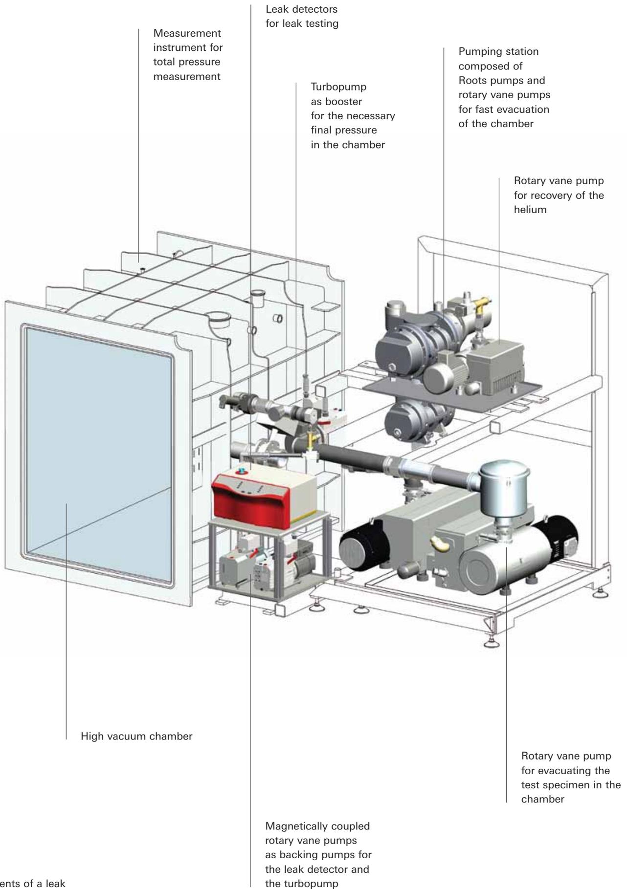
Components of a leak testing system from a single source
