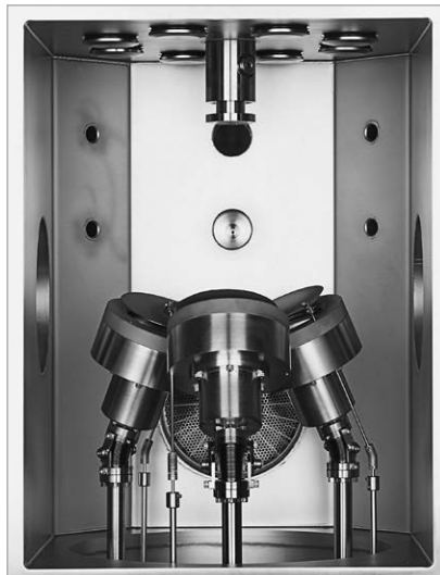
Confocal arrangement of 3-in. sputter sources, aligned for sputter-up
