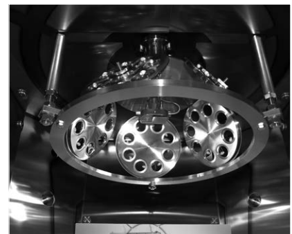
Planetary drive with central friction disc and five free-running planets
