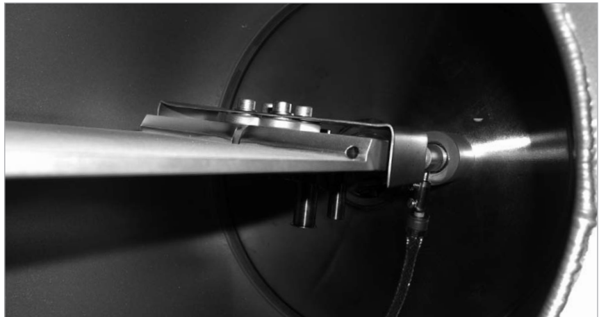
Insulated substrate fork with RF bias connection
