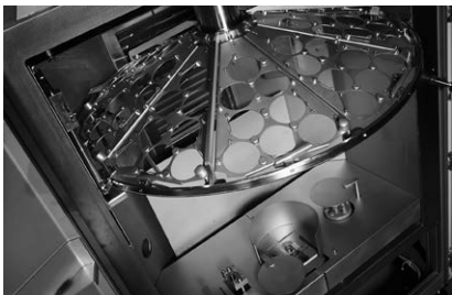
Chamber bottom: electron beam evaporator, thermal evaporator, ion source Chamber top: rotating substrate dome with turnover device
