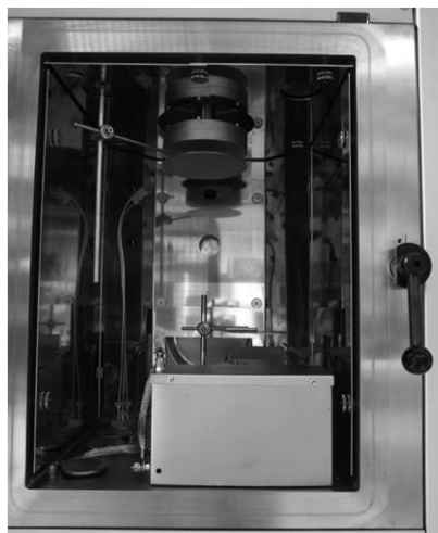
Rotating and water-cooled substrate table
