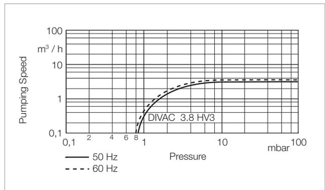
Pumping speed curve of the DIVAC 3.8 HV3
