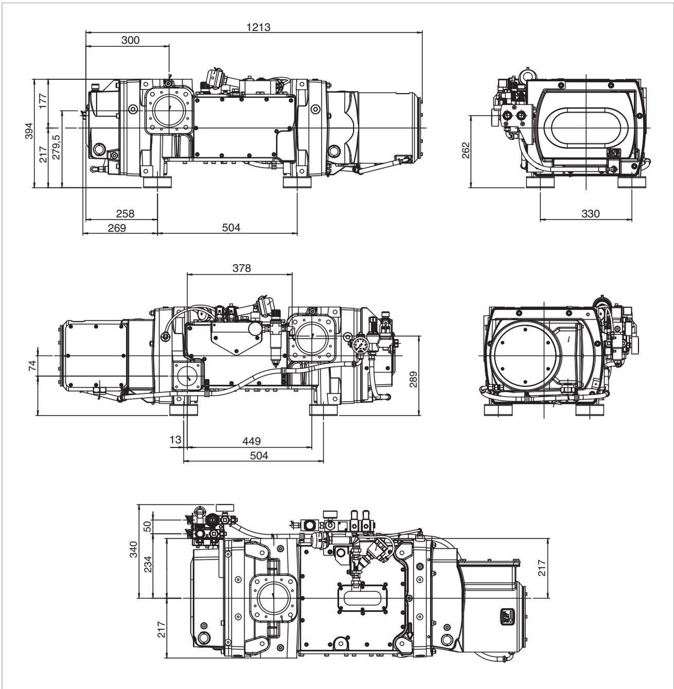
Dimensional drawing for the DRYVAC DV 450-r and DV 650-r
