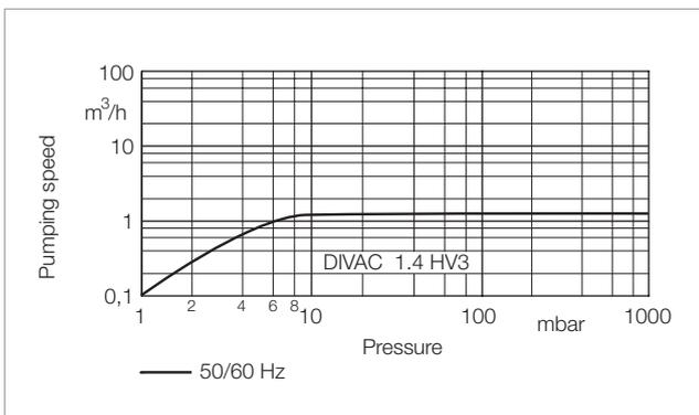
Pumping speed curve of the DIVAC 1.4 HV3
