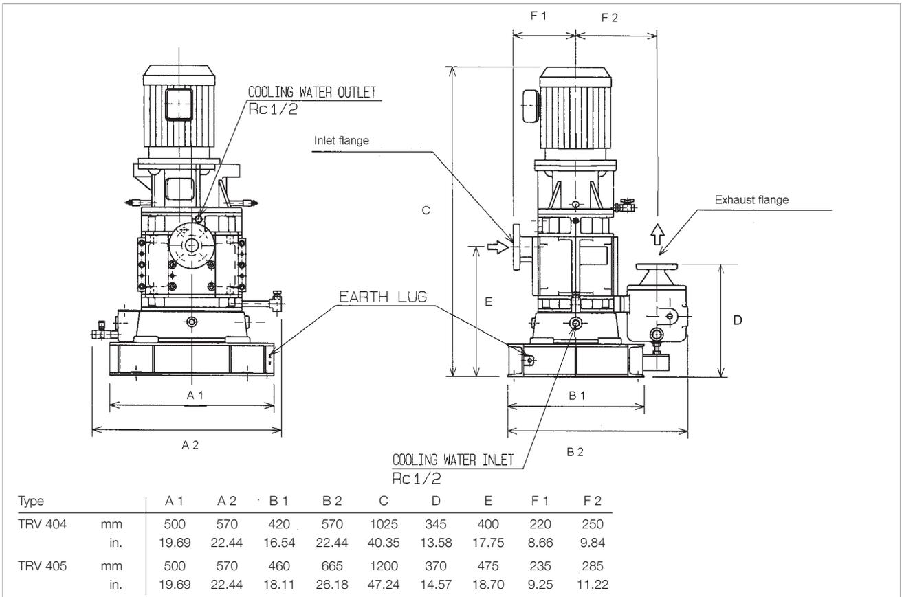
Dimensional drawing of the CHEMROVAC TRV 404 and 405
