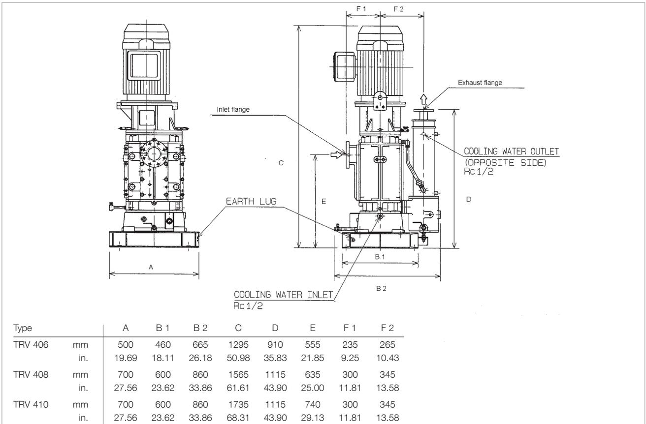
Dimensional drawing of the CHEMROVAC TRV 406 to 410
