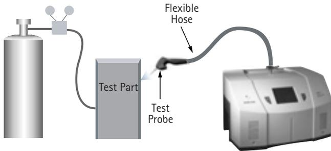
Figure 4 Locating Leaks – Inside Out
