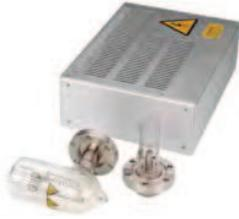
The Edwards Ion Gauge Controller (IGC) provides all the power, control and signal conditioning required to run one or two ion gauge heads. When connected to a Edwards TIC Instrument Controller the user has full control of the ion gauge functions from the TIC front panel. This includes features such as automatic emission current selection and interlock with other gauge types.
