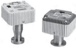
A compact Active ion gauge with dual yttria coated iridium filaments, a wide measuring range from  $6.6 \times 10^{-2}$  to  $6.6 \times 10^{-10}$  mbar ( $5 \times 10^{-2}$  to  $5 \times 10^{-10}$  Torr) and a 1 Volt/decade linear output.
