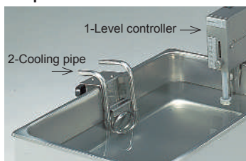
1-Level controller 2-Cooling pipe
