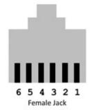
The pins are numbered looking into the female connector with the pins on the bottom from right to left. Note that the first two pins are signals coming from the Digital 300 to the bus master while the last two pins are signals coming to the Digital 300 from the bus master.
