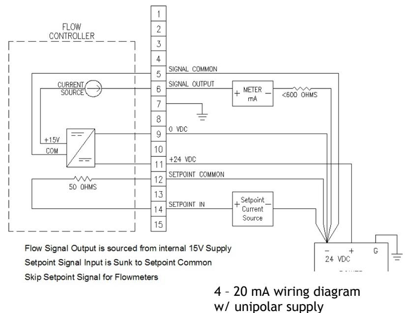
Besides the standard input lines, controller versions have a valve override input available on pin 8 referenced to pin 5. If pin 8 is allowed to float, the valve is controlled internally. If a voltage above 2.4 VDC is placed on pin 8 with respect to pin 5, the valve will open fully. If a voltage below 0.4 VDC is placed on pin 8, the valve will close. Care should be taken to ensure this voltage remains between -16 and +16 VDC.
