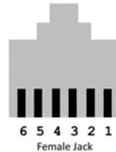
The pins are numbered looking into the female connector with the pins on the bottom from right to left. Note that the first two pins are signals coming from the Digital 300 to the bus master while the last two pins are signals coming to the Digital 300 from the bus master.
