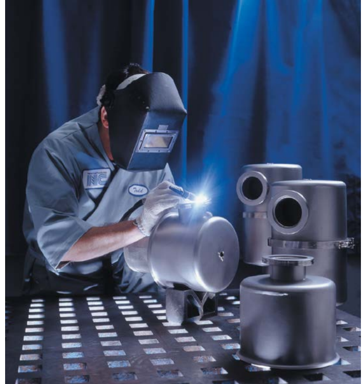
TIG Fusion Welding
