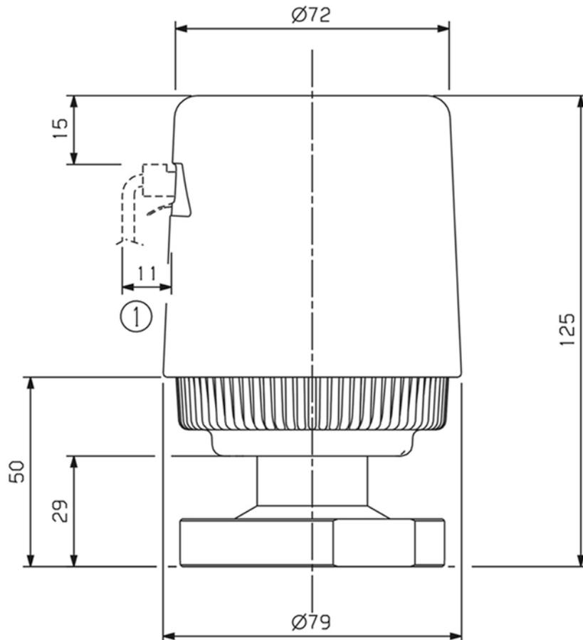
1. Clearance required for electrical cable
