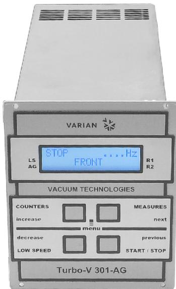
The Turbo-V 301-AG Rack controller is a microprocessor-controlled frequency converter with new, enhanced features that allow greater control and communication capabilities. This compact, 1/4 rack unit is designed for full worldwide compatibility, for vent valve control, active gauge pressure reading and pump operation parameters control, as well as for self diagnostic and protection features.
