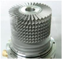
*Aluminum rotor with EDM bladed stages*
