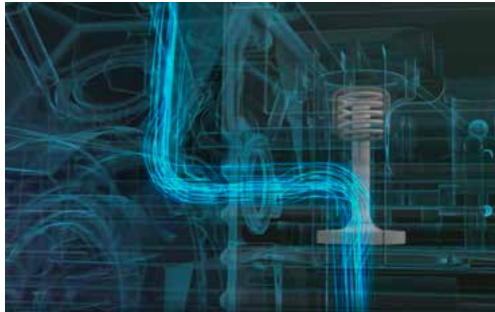
Vacuum safety valve open
