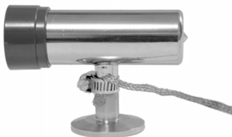
Figure 2-8 Convectron Gauge to Vacuum Chamber Ground Connection
