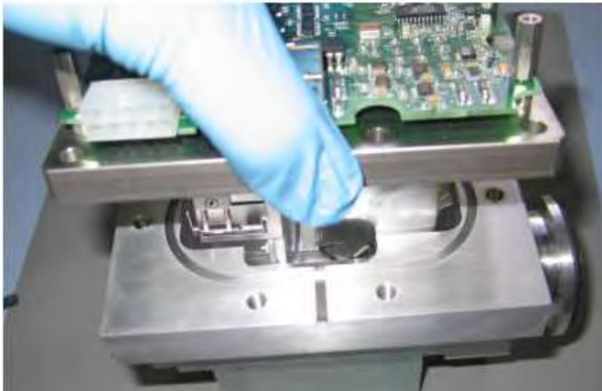
**Figure B-52 Spectrometer Assembly Removal**
