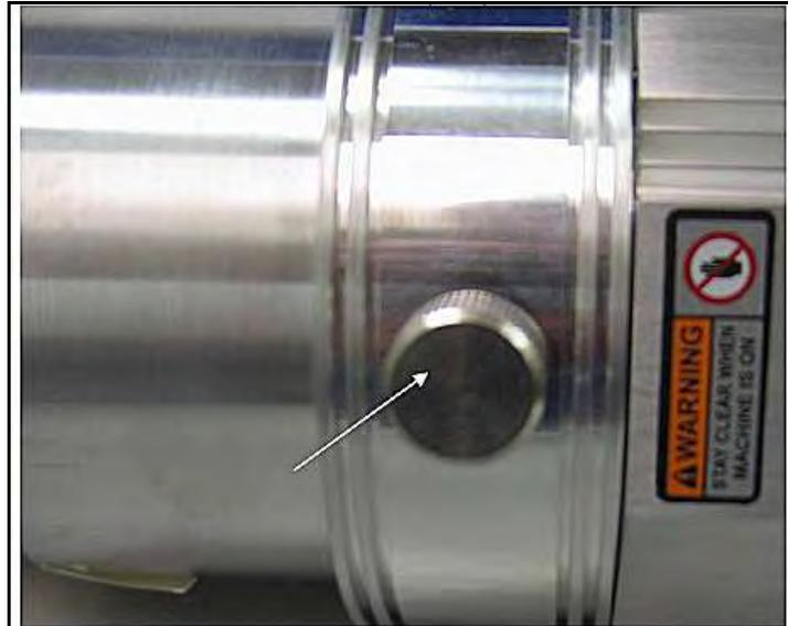
**Figure B-15 Turbo Pump Vent Screw**
