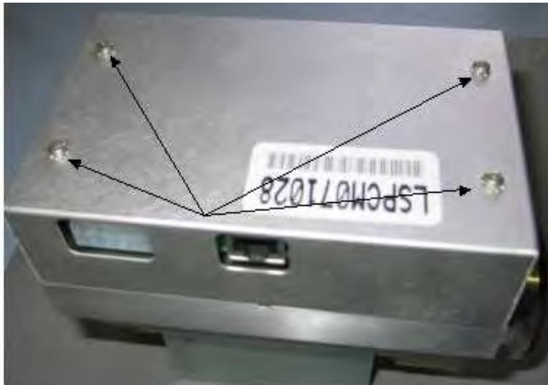
**Figure B-61 Spectrometer Cover Screws**
