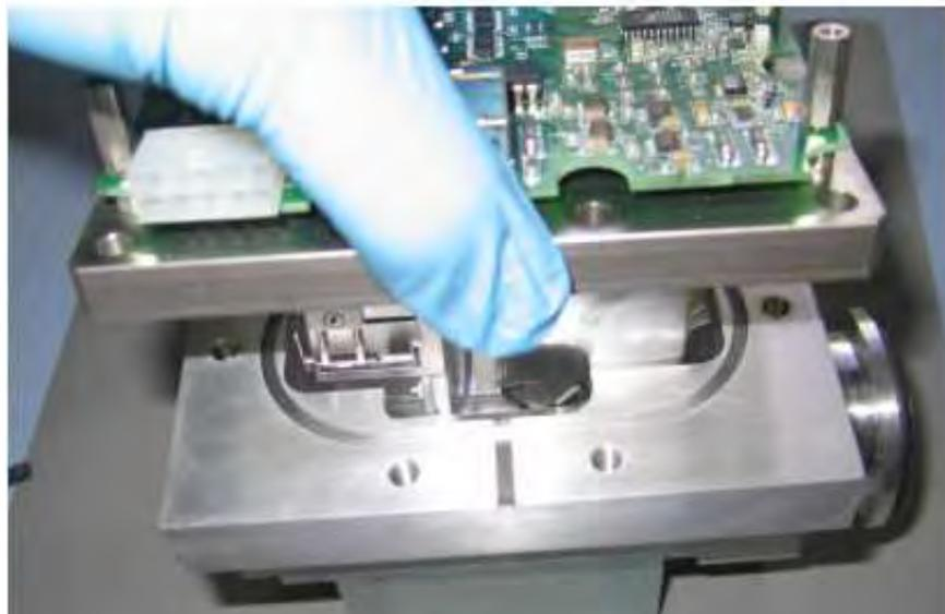
**Figure B-63 Spectrometer Assembly Removal**
