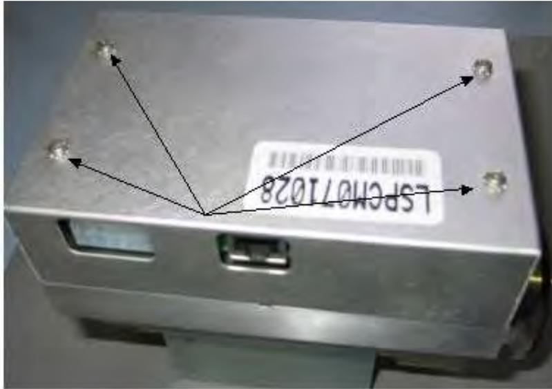
**Figure B-78 Spectrometer Cover Screws**
