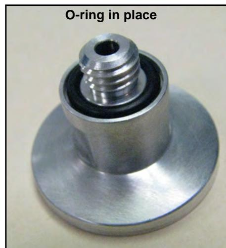
**Figure B-17 Turbo Pump Flange in Place**
