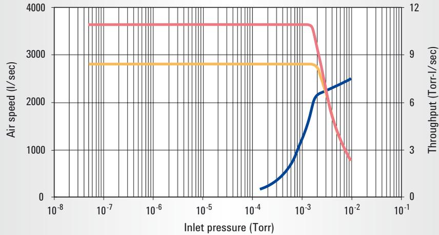
— Pumping speed/Standard cold cap      — Pumping speed/Extended cold cap      — Throughput
