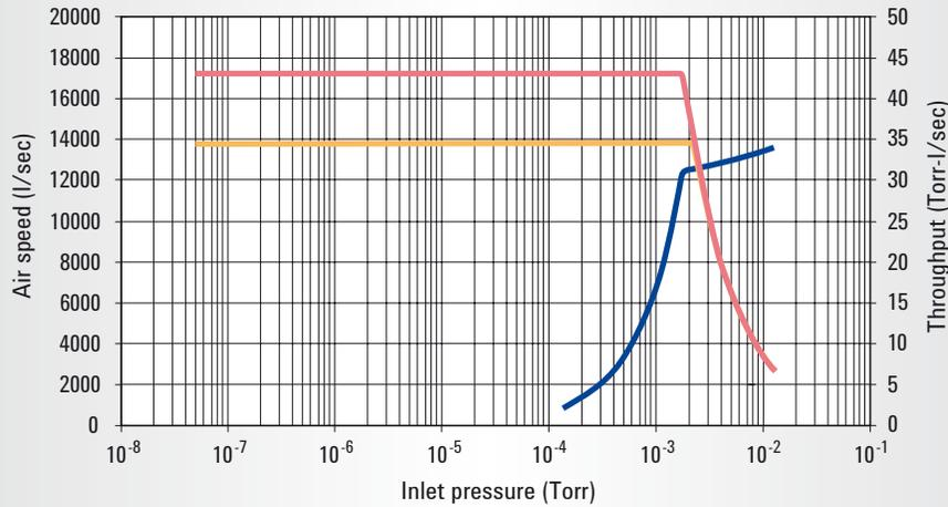
— Pumping speed/Cold cap      — Pumping speed/Halo baffle      — Throughput
