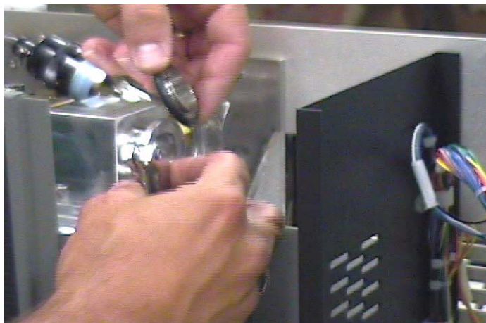
Figure 3-18 Spectrometer Tube O-ring and Centering Ring
