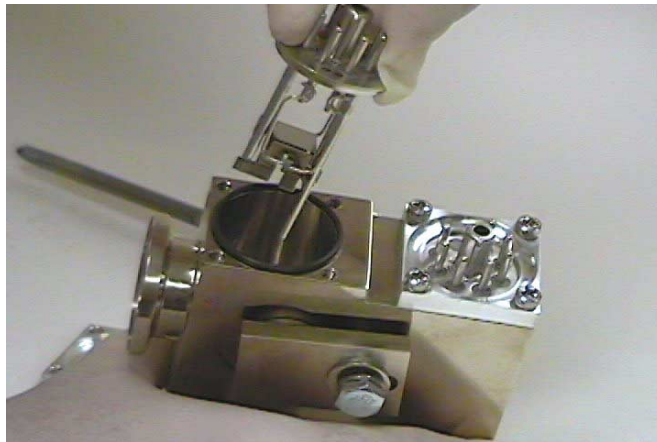
Figure 3-9 Removing the Ion Source
