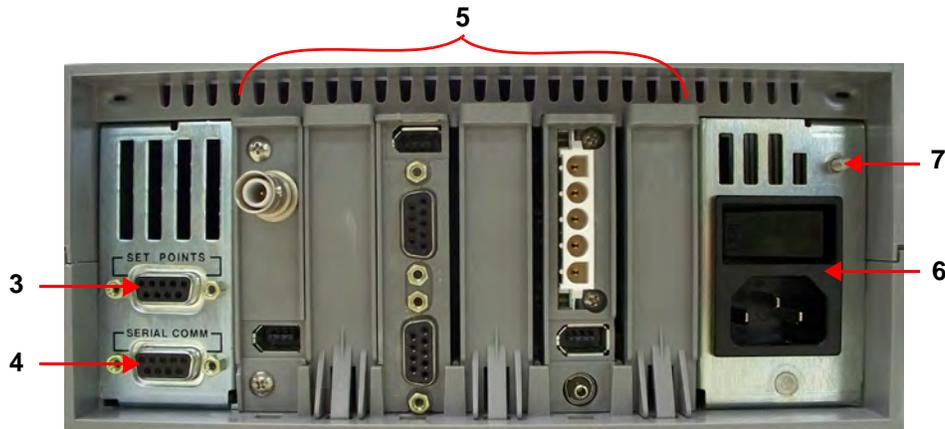
Figure 1-2 Backplate Connections
