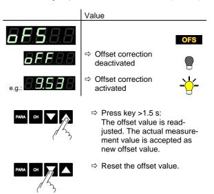
When the offset correction is activated, the saved offset value is subtracted from the actual measurement value. This allows measuring relative to a reference pressure.
