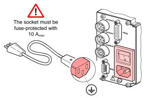
If the unit is installed in a switching cabinet, the mains voltage should be supplied and turned on via a central distributor.
