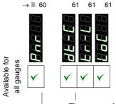
The name of the parameter is displayed as long as the key is pressed or at least for 1.5 s.
