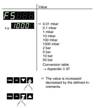
Offset correction The offset value is displayed and readjusted according to the actual measurement value (in the range of
