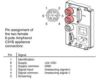
**3.5** *control* **Connector** This connector allows to read the measuring signal, to evaluate the state of the floating contacts of the error relay, and to activate or deactivate the gauges ( $\rightarrow \square 47$ ).
