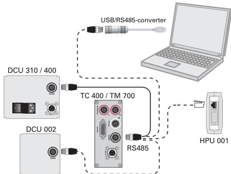
Fig. 3: Optional connection possibilities for interface RS485
