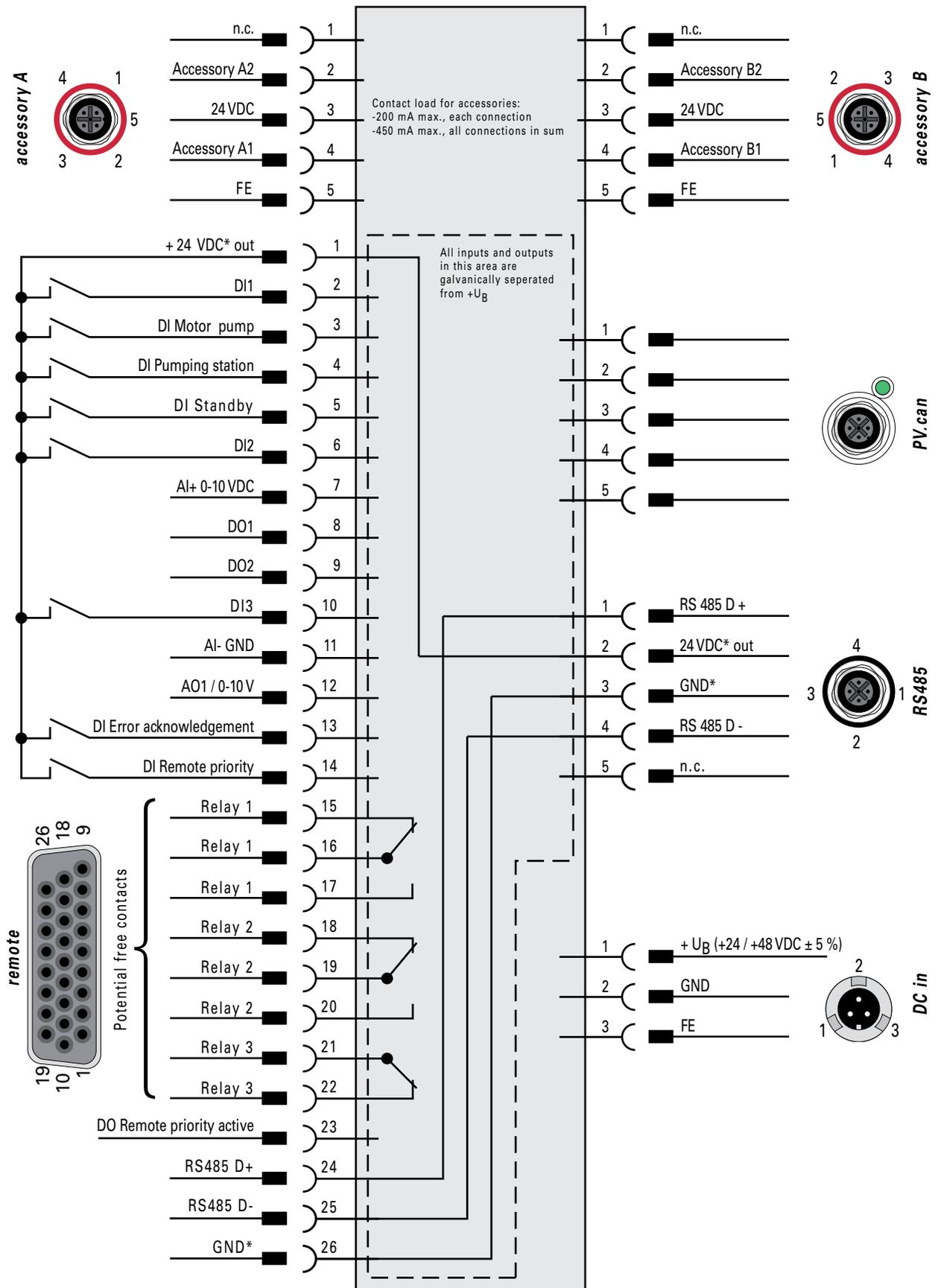
Fig. 2: Connections diagram and assignment of the TC 400
