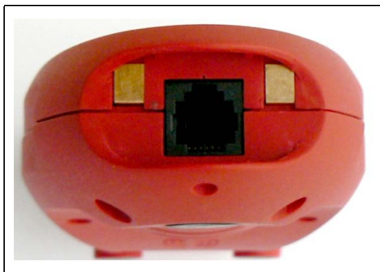
Fig. 5 RJ25 socket on the bottom of the remote control
