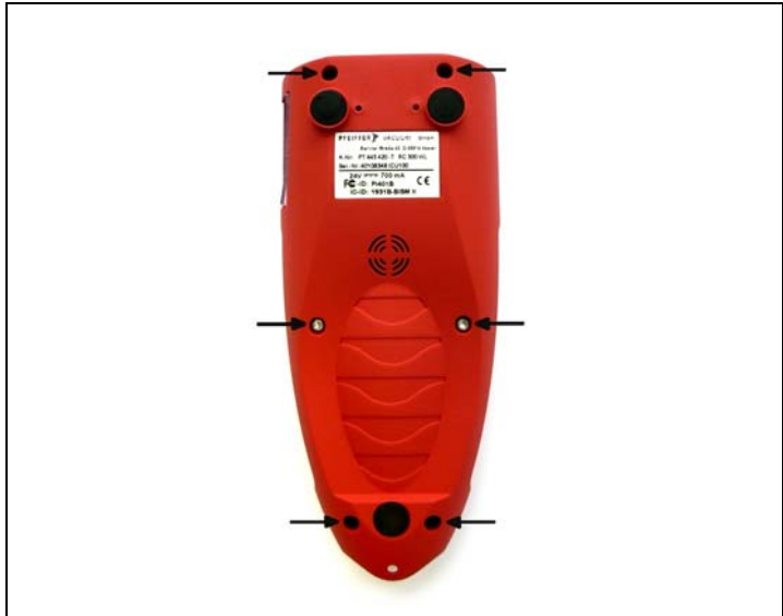
Fig. 29 Screws on the bottom of the remote control
