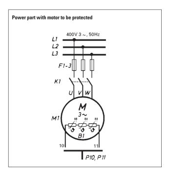
Use a tripping unit with error signal storage, e.g. a PTC tripping unit with two switchover contacts at the output (see Section 9. Accessories).
